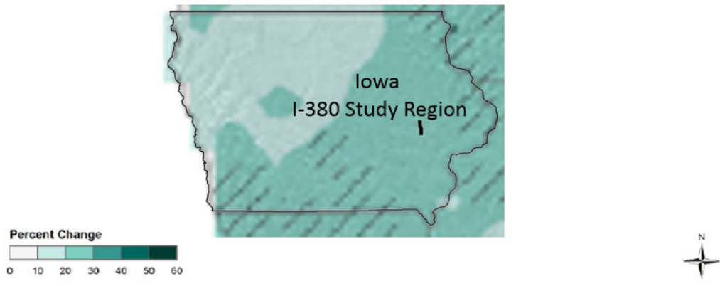
Figure A-20. MIDWEST REGION SIMULATED DIFFERENCE IN THE MEAN ANNUAL NUMBER OF DAYS WITH A MAXIMUM PRECIPITATION GREATER THAN 1 INCH, FOR THE 2041-2070 TIME PERIOD IN REFERENCE TO 1980-2000 FOR THE NARCCAP MULTI-MODEL MEAN HIGH EMISSIONS SCENARIO.
