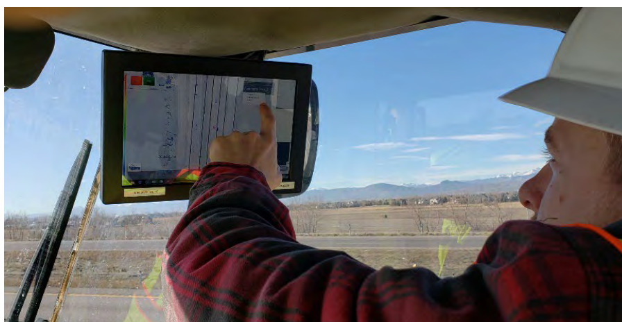
Figure 14. Machine operator interacting with on-board Comp-Score RT display.
