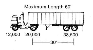
The 58,500 pounds on the group of axles is within the maximum weight limit shown on the attached table for a group of axles having a distance of 30 feet. The gross weight of 70,500 pounds is within the 80,000 pound limit, and the weight on the single axles is within the 20,000 pound limit. But, the 38,500 pounds is in excess of the 34,000 pound limit on a tandem axle. If the vehicle is not transporting livestock there is clearly a violation of §321.463, 1981 Code of Iowa on the tandem axle.
