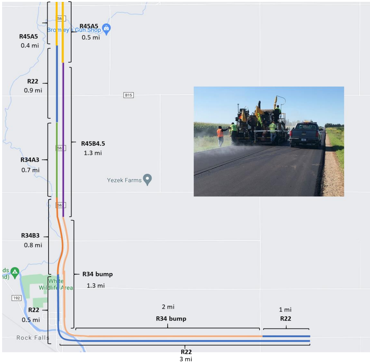
Figure 7-1. Construction of Six Test Sections in Cerro Gordo County
