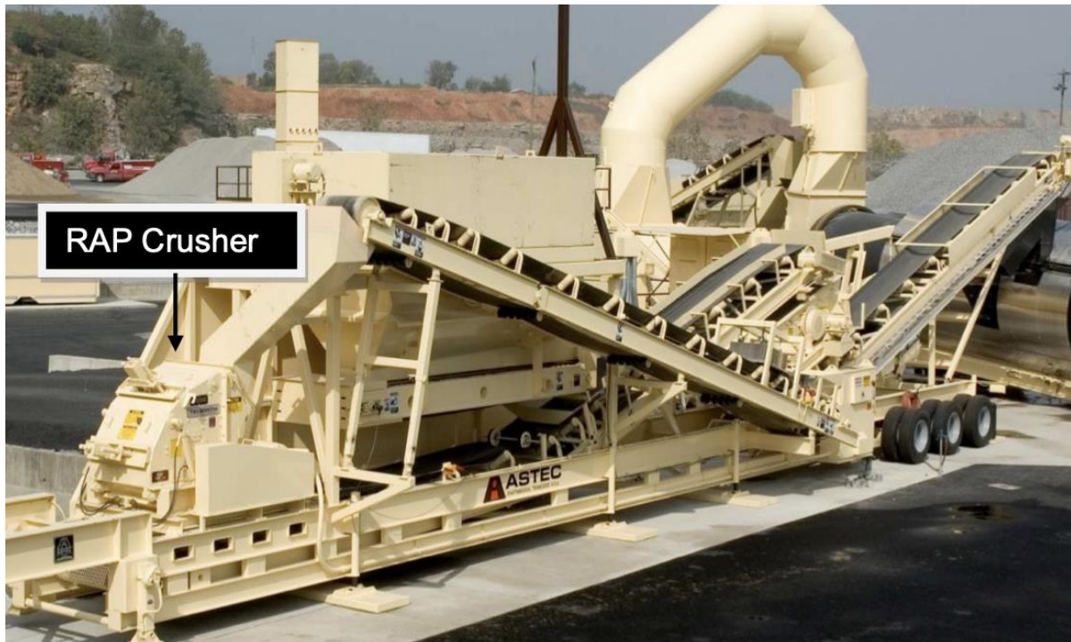
Figure 3-5. RAP processing unit with a screen before the crusher (West et al. 2016)
