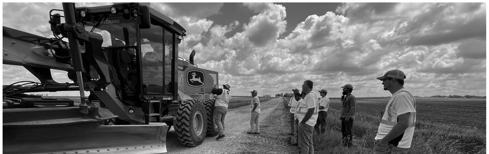
**Wyatt Nelson, left, from Murphy Equipment, demonstrates how to access the motor grader's engine compartment as part of the pre-trip inspection process at the MoGO Field Days on-site training in Ames**
