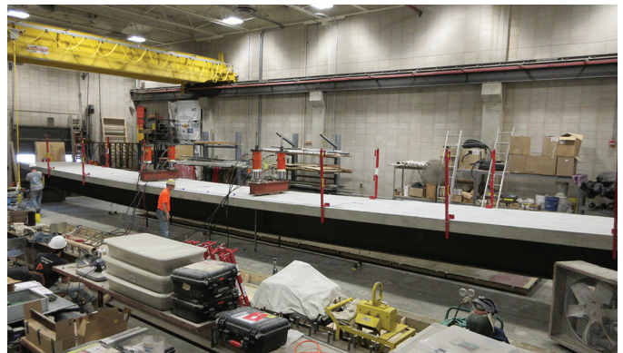
Full-scale W30×173 composite beam test setup in the laboratory
