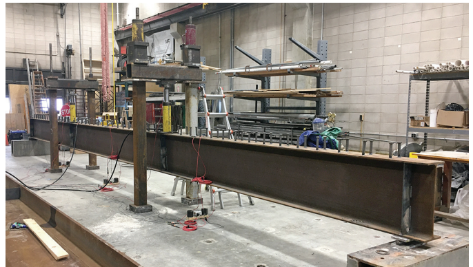
Full-scale W24×68 non-composite load test setup in the laboratory
