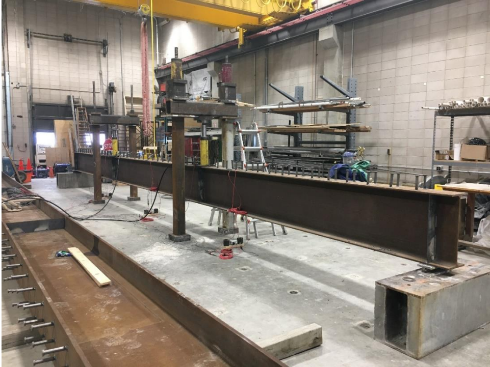
Figure 9. W24×68 non-composite load test
