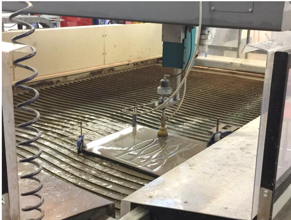
Figure 35. Fatigue sample water-jet cutting
