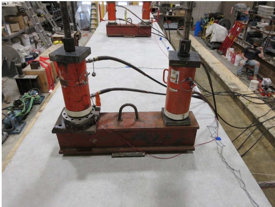
Figure 24. W30×173 composite beam load actuators
