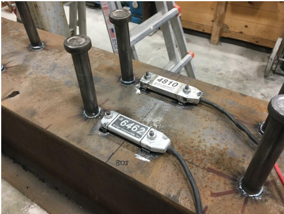
Figure 12. Strain gauges on non-composite beam
