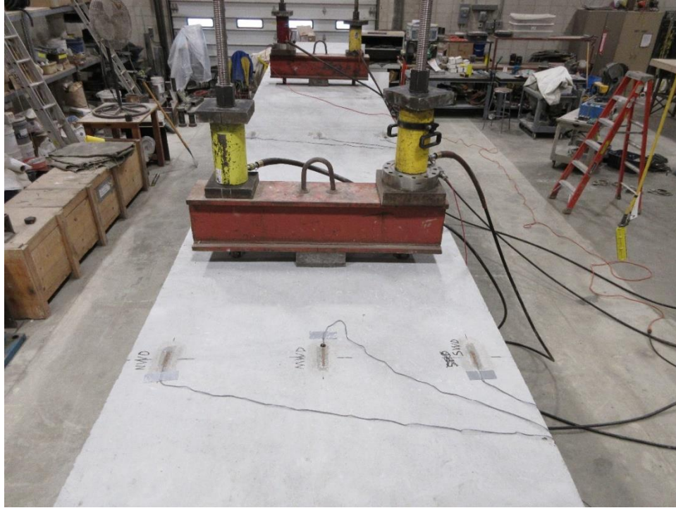
Figure 23. W24×68 composite beam load actuators
