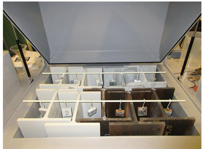
*Pile specimens and coupon samples inside the cyclic corrosion chamber*
