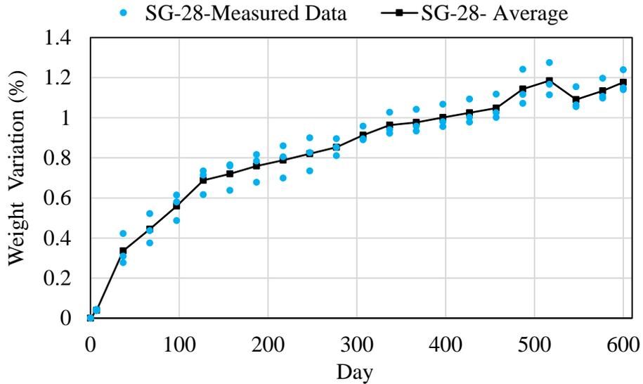
**Figure 12. Weight variation (%) of SG-28 samples**
