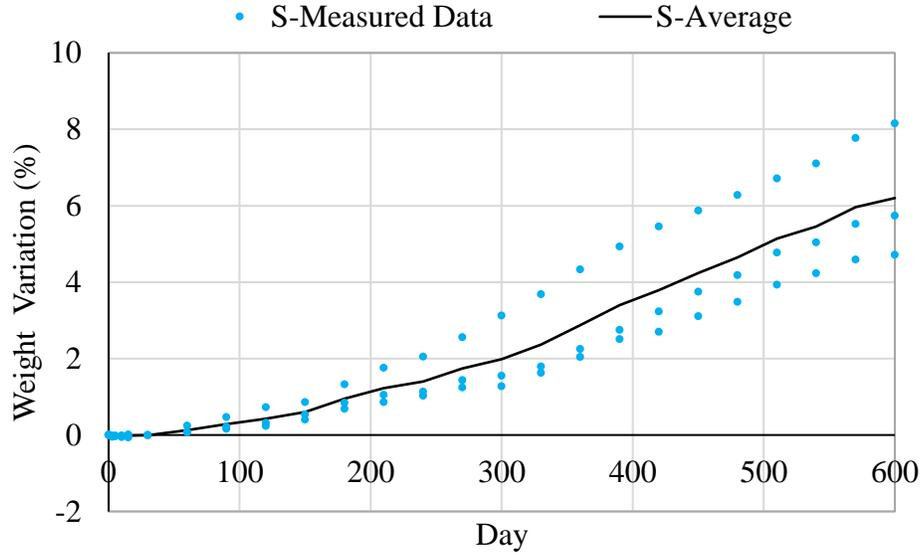
**Figure 5. Weight variation (%) of samples without coating**
