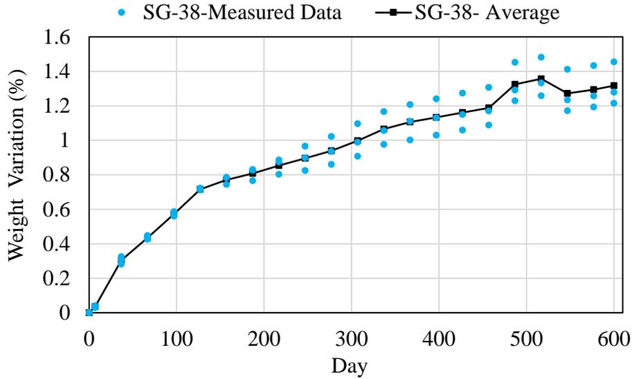
**Figure 13. Weight variation (%) of SG-38 samples**
