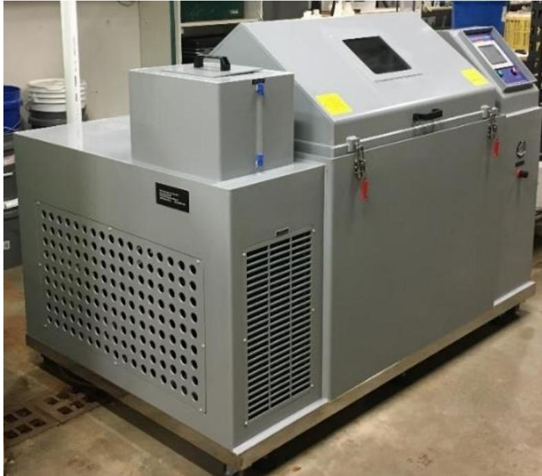
**Figure 2. Cyclic corrosion test chamber**
