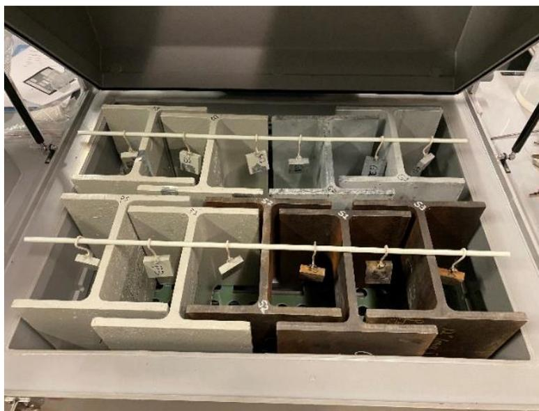
**Figure 4. Samples inside the cyclic corrosion chamber**
