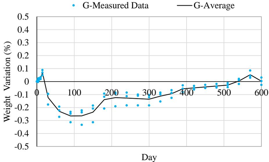
**Figure 8. Weight variation (%) of samples with galvanized coating**
