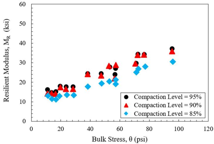
**Figure 15.** Resilient modulus ( $M_R$ ) test results for US-13 (RPCC)
