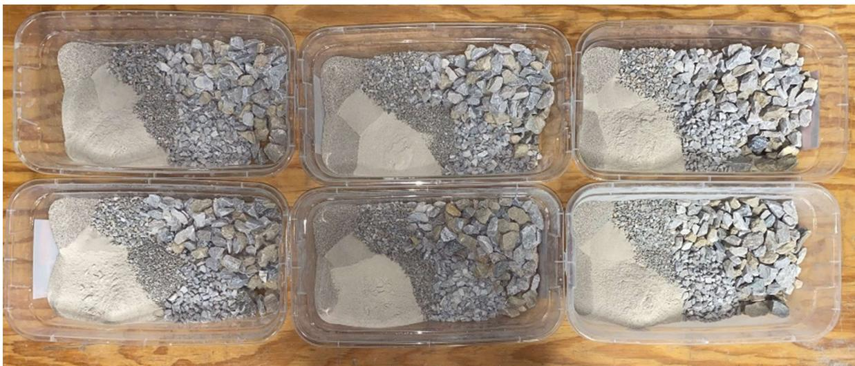
**Figure 11.** Materials prepared for each lift of one prismatic specimen for resilient modulus ( $M_R$ ) testing
