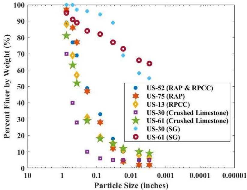
**Figure 1.** Particle size distributions of materials (RAP = reclaimed asphalt pavement; RPCC = reclaimed Portland cement concrete; SG = subgrade)
