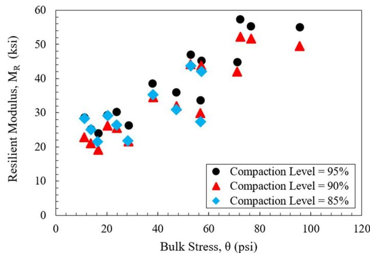
**Figure 13.** Resilient modulus ( $M_R$ ) test results for US-52 (RAP & RPCC)
