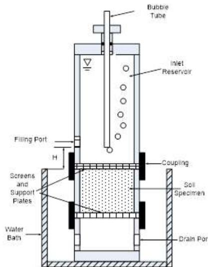
**Figure 7.** Bubble tube constant head permeameter
