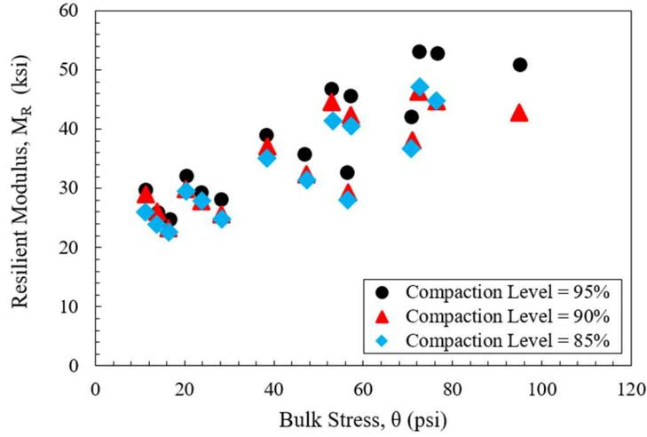
**Figure 14.** Resilient modulus ( $M_R$ ) test results for US-75 (RAP)
