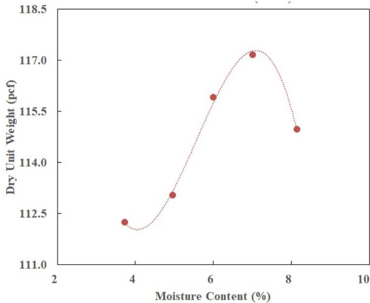
**Figure 3.** Compaction curve for US-75 (RAP)
