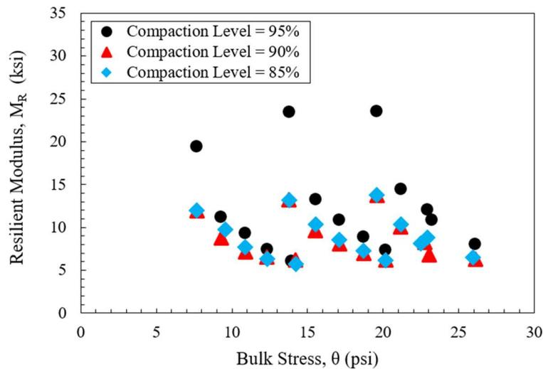
**Figure 17.** Resilient modulus ( $M_R$ ) test results for US-61 (SG)
