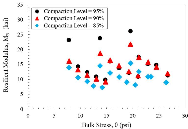
**Figure 16.** Resilient modulus ( $M_R$ ) test results for US-30 (SG)
