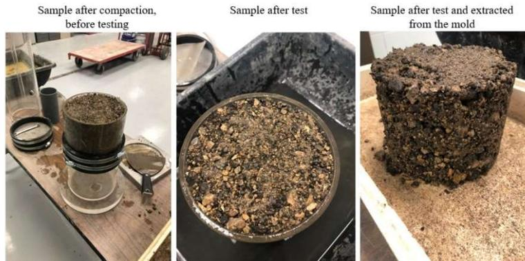
**Figure 8.** Specimens prepared from US-52 (RAP & RPCC) at (a) 95, (b) 90, and (c) 85% compaction levels
