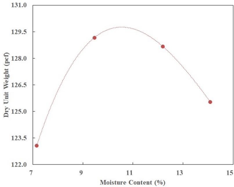
**Figure 5.** Compaction curve for US-30 (SG)
