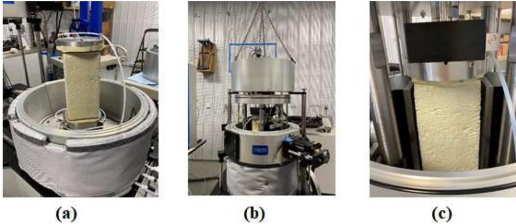
**Figure 12.** Specimen assembly for resilient modulus ( $M_R$ ) testing: (a) specimen attached to the bottom and top platens, (b) specimen in the testing chamber, and (c) specimen attached to the vertical load actuator
