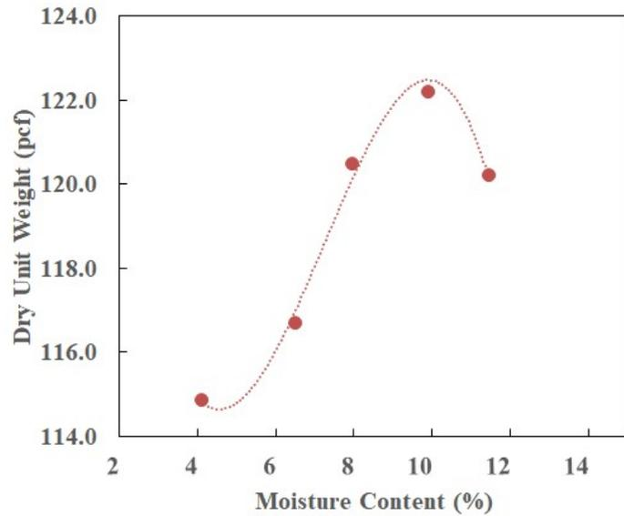
**Figure 2.** Compaction curve for US-52 (RAP & RPCC)
