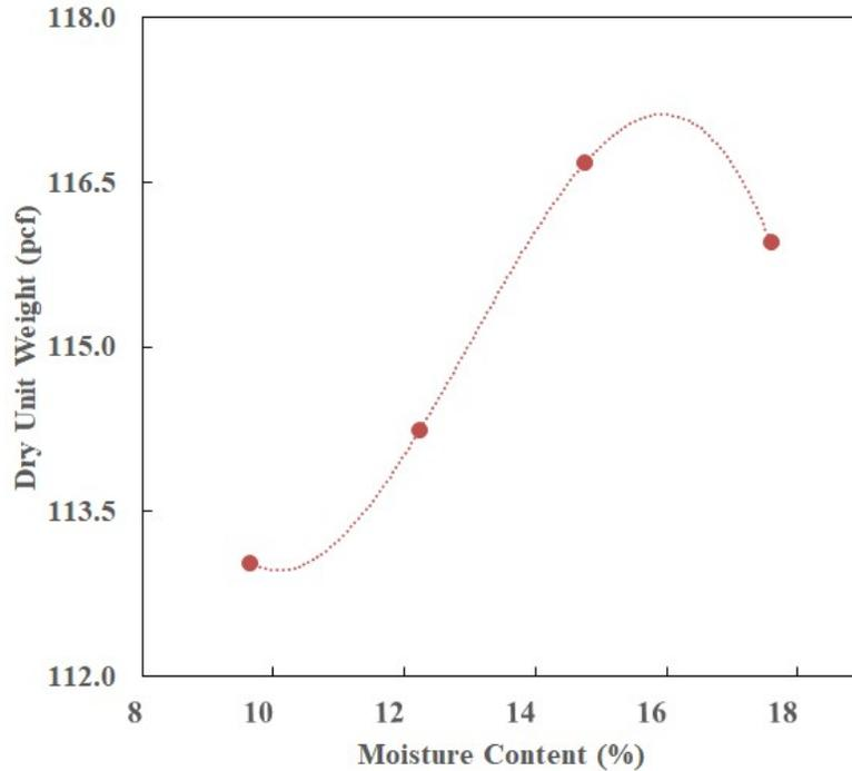
**Figure 6.** Compaction curve for US-61 (SG)
