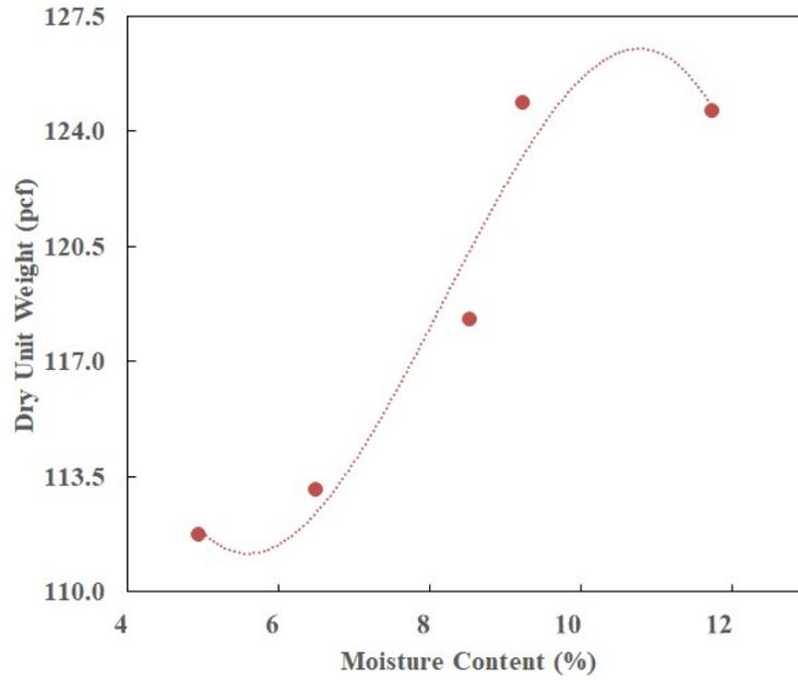
**Figure 4.** Compaction curve for US-13 (RPCC)
