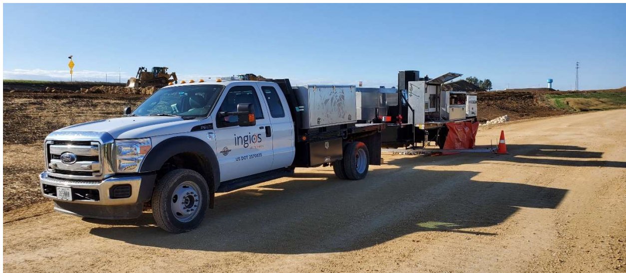
Figure 2. Automated Plate Load Testing trailer.
