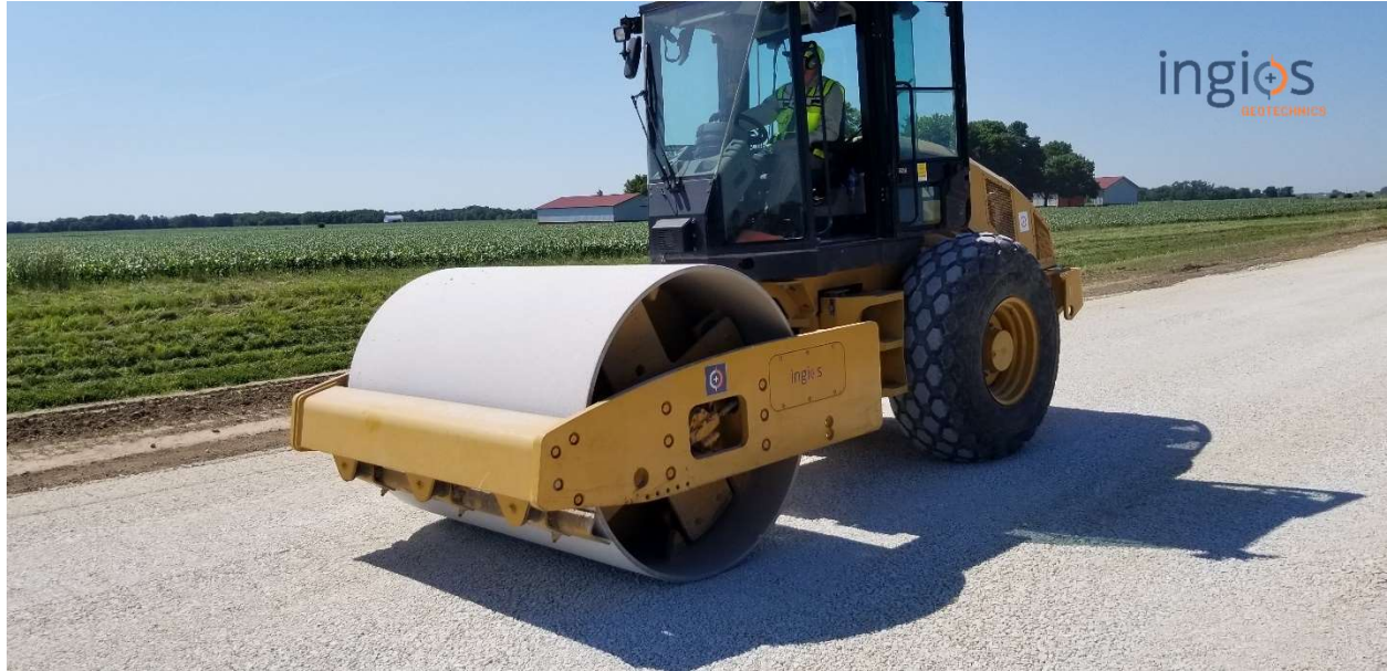
Figure 1 .Caterpillar CS56 vibratory smooth drum roller outfitted with Ingios COMP-Score RT system and GPS.
