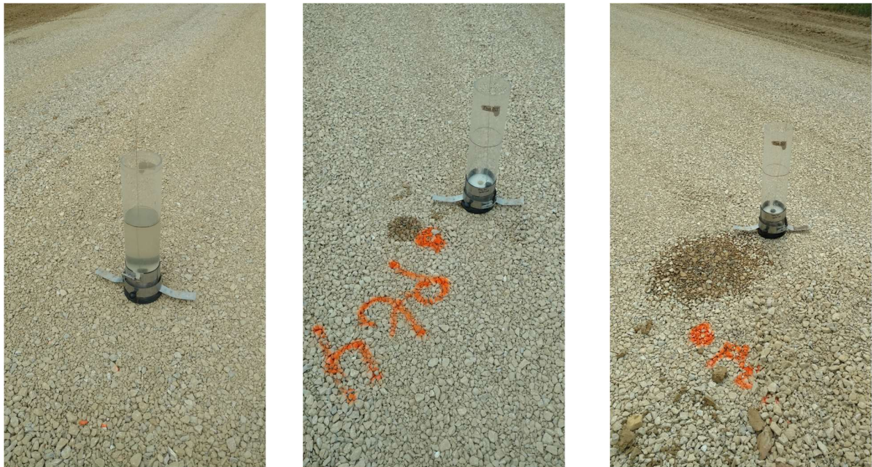
Figure 17. Vu meter testing on crushed limestone granular subbase on Tama County US30 (07/09/2020).
