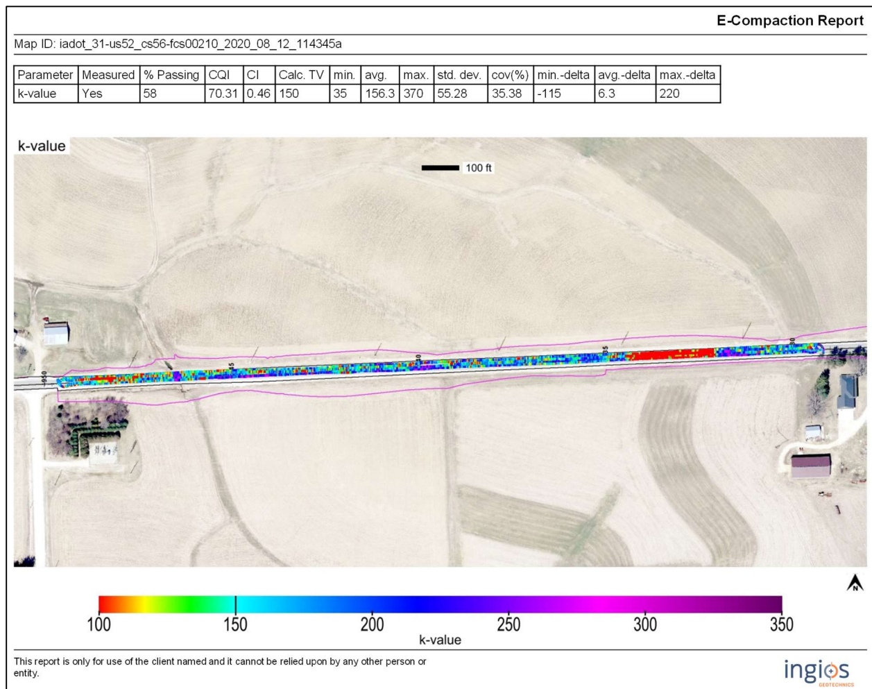
Figure 5. Sample compaction map page showing k-value data overlaid on aerial imagery.
