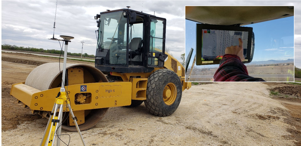
Figure 2. Vibratory smooth drum roller outfitted with modulus-mapping technology (insert: touch screen monitor for selection and viewing of results in real-time).
