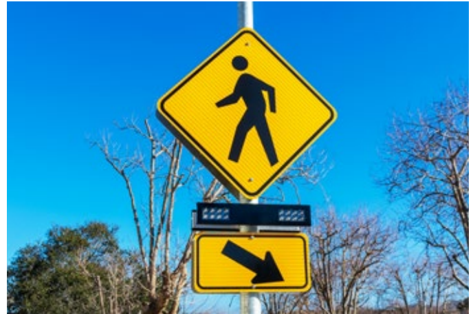
Figure 2.11: Rectangular rapid flashing beacon
