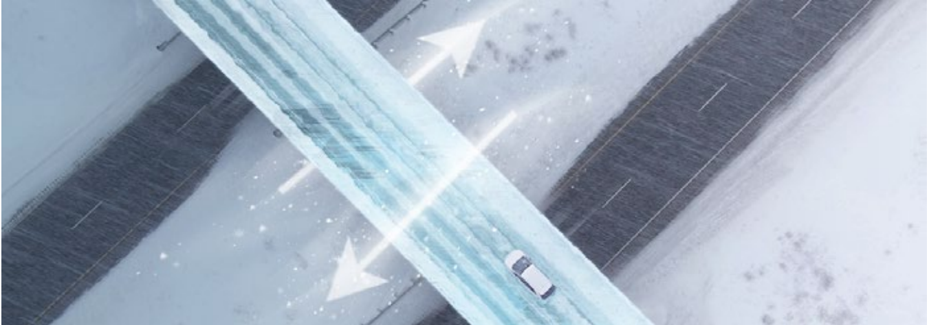
Figure 5.9: Ice forms on bridges first due to circulating air both above and below the road surface.
