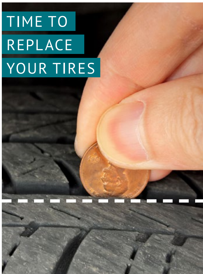
Figure 3.1: Check your tire tread with a penny
