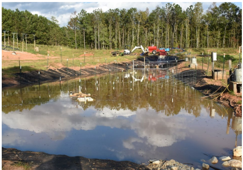
Most Feasible and Effective Installation (MFE-I) during sediment-laden flow introduction
