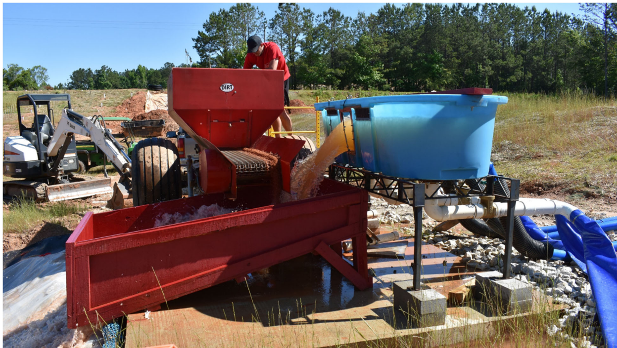
Figure 3.9. Flow and sediment introduction system.
