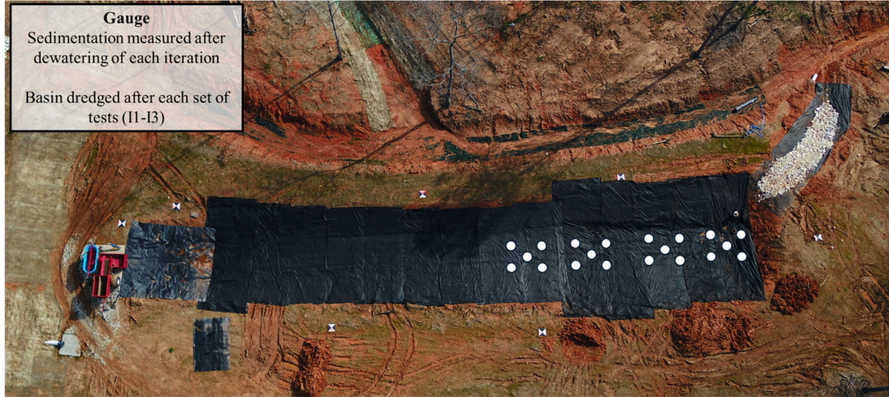
Figure 3.15. Sedimentation gauge configuration.
