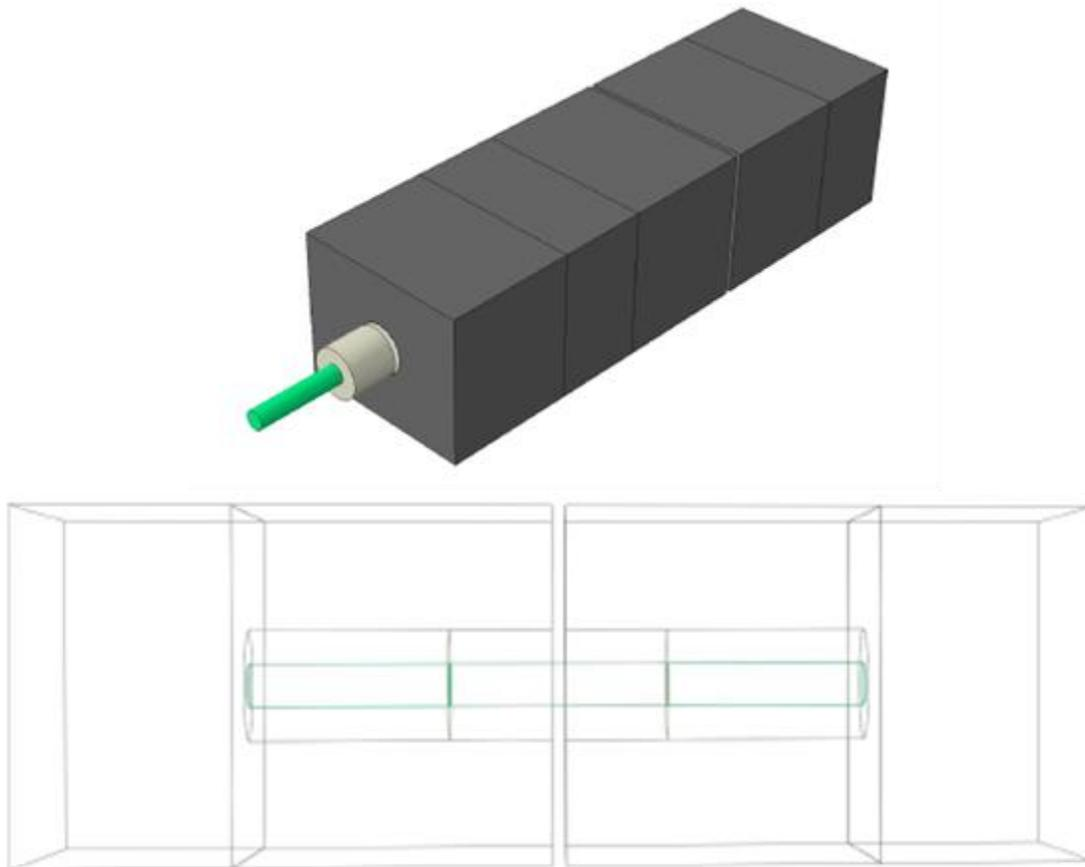
**Figure 13. Isometric and plan view drawings of ABAQUS models showing model components for AASHTO T 253 test configuration (top drawing shows right  $\frac{2}{3}$  of full specimen; bottom shows  $\frac{1}{2}$  of full specimen)**
