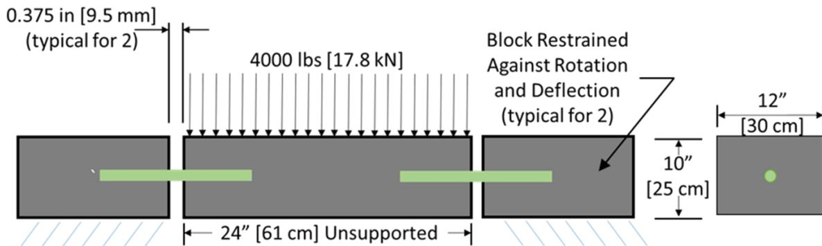
**Figure 1. Schematic of AASHTO T 253 load-deflection test for concrete pavement dowels, with relative deflection limited to 10 mils (0.01 in.) [0.25 mm]**
