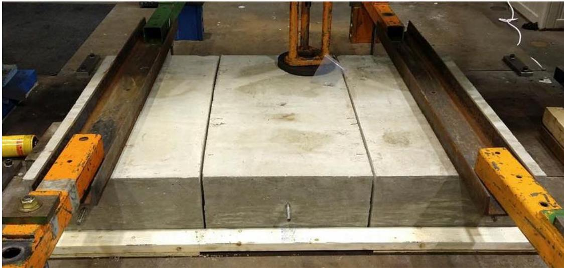
**Figure 17. Photo of modified AASHTO T 253 test setup in CTLGroup laboratory**
