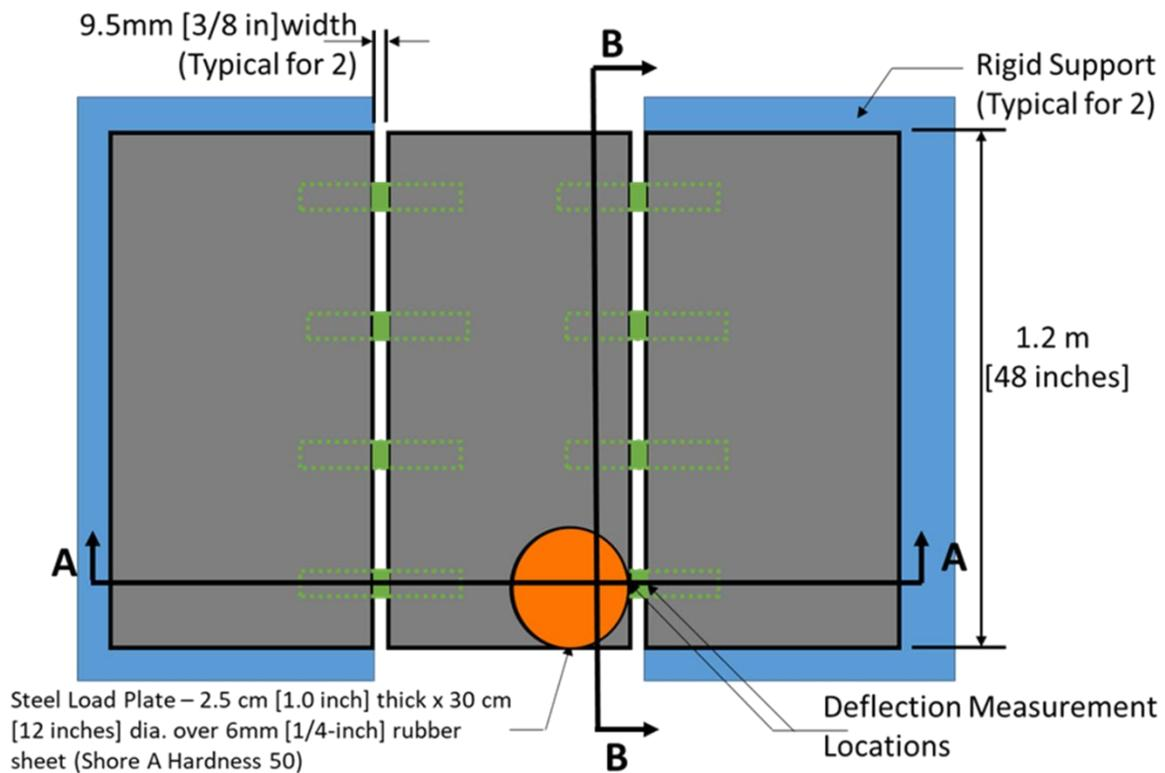
**Figure 2. Proposed modified AASHTO T 253 dowel load-deflection test – plan view**
