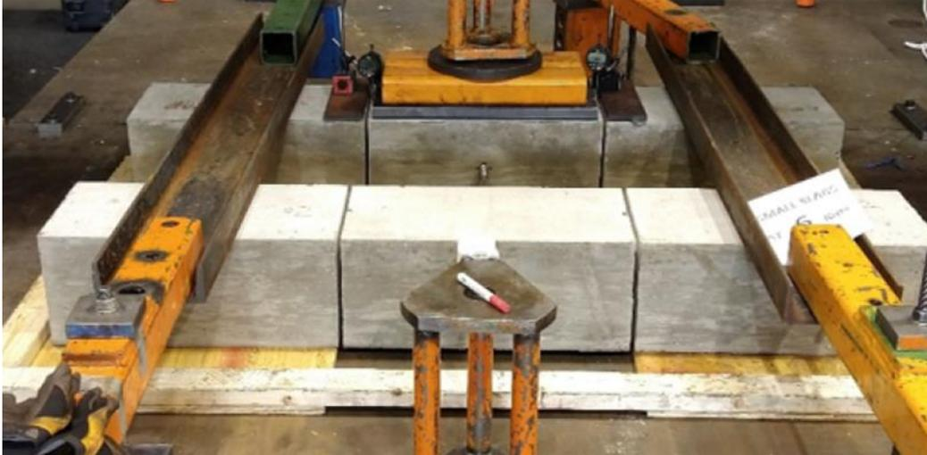
**Figure 16. Photo of AASHTO T 253 test setup in CTLGroup laboratory**
