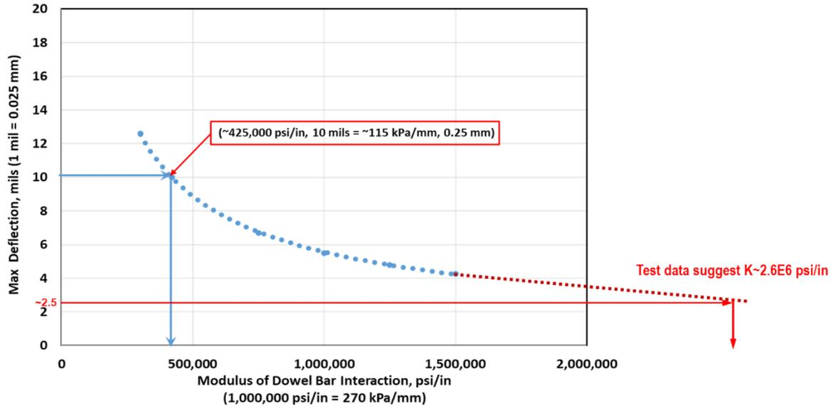
**Figure 8. Extrapolation of Figure 5 data to estimate experimental K for AASHTO T 253 load-deflection test**
