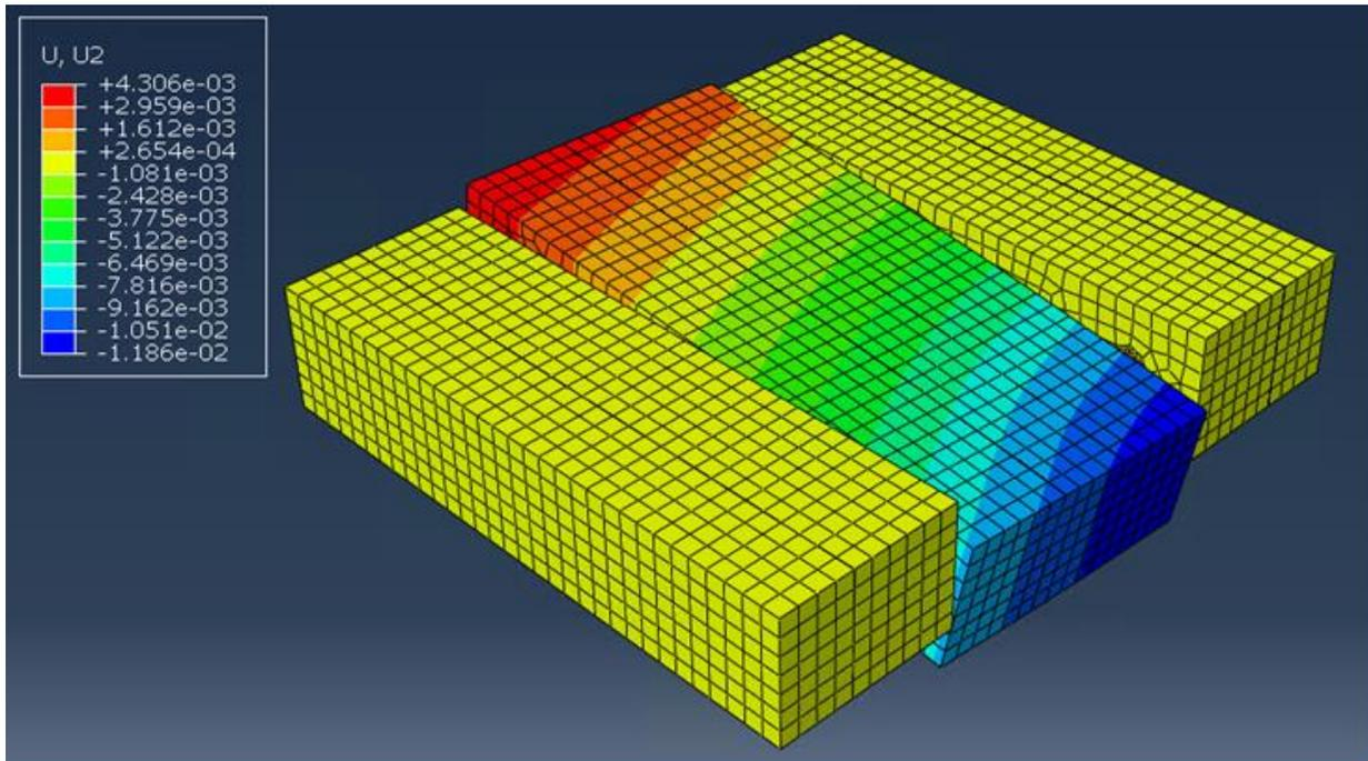
**Figure 11. ABAQUS model of slab deflections for modified AASHTO T 253 test under 9,000 lb corner load**
