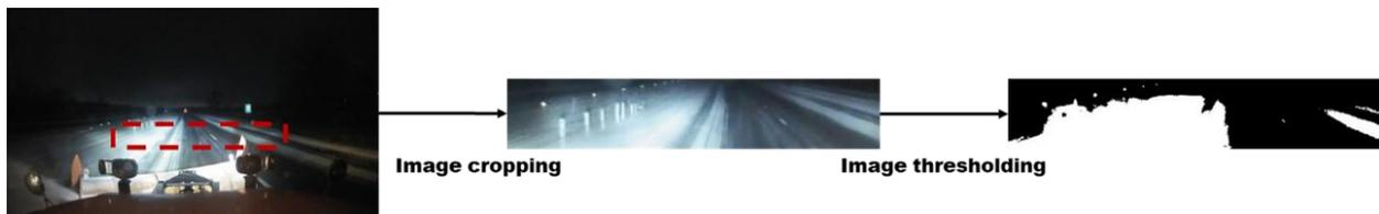
**Figure 4-4. Example of image cropping and thresholding process**
