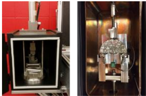
Figure 1. I-FIT SCB test, left, and AASHTO TP 105-13 SCB test, right
