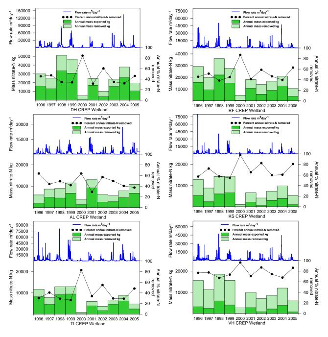
Figure 3. Predicted annual nitrate-N loading and loss rates for selected wetlands in the Iowa CREP service area for 1996 to 2005 input conditions.
