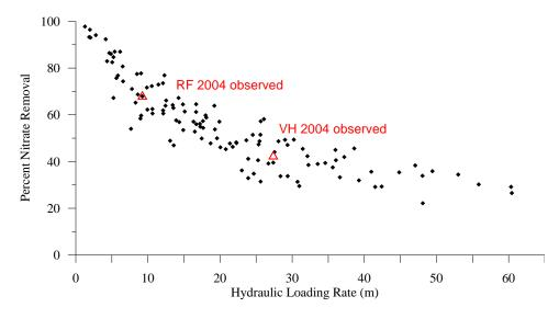
Figure 4. Modeled percent nitrate removal for 1996 to 2005 input conditions.
