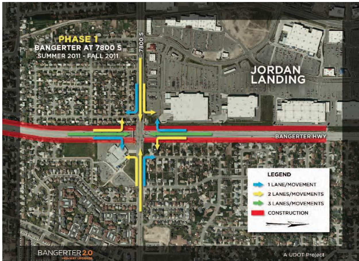
Figure C.2.1.2 Traffic movements for Phase 1 construction of SPUI at Bangarter Highway and 7800 South
