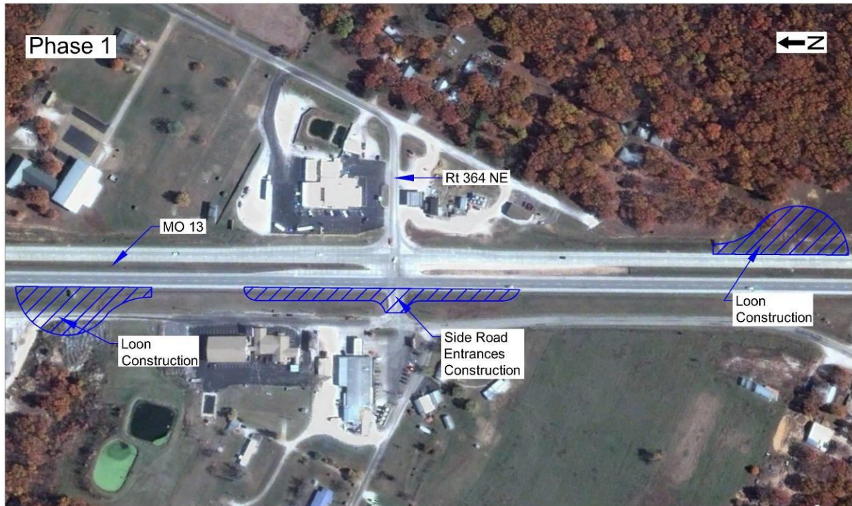
Figure C.4.1.2 Phase 1 construction of RCUT at MO 13 and Route 364 NE
