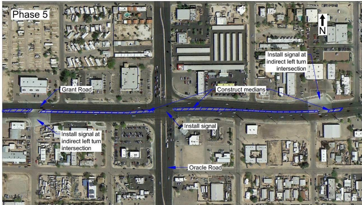
Figure C.5.1.6 Phase 5 construction of MUT at Grant Road and Oracle Road
