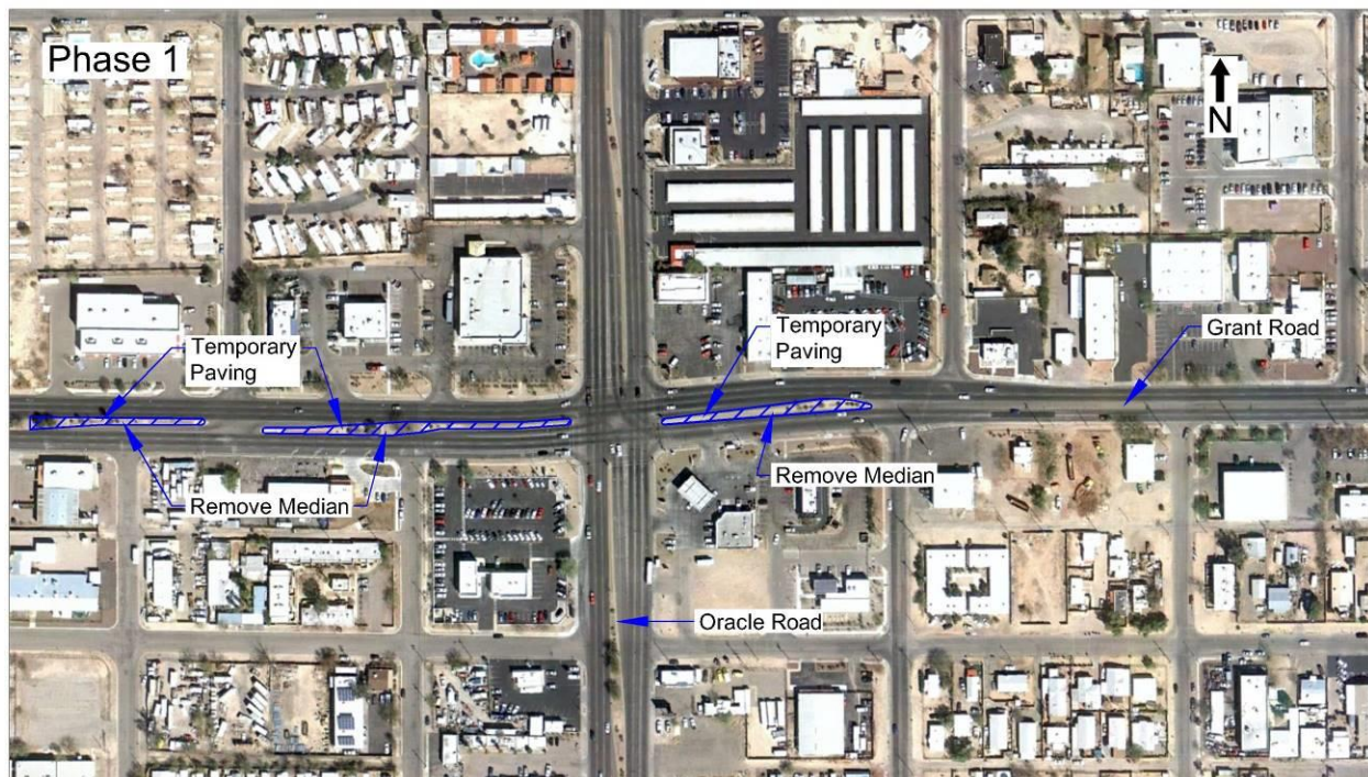
Figure C.5.1.2 Phase 1 Construction of MUT at Grant Road and Oracle Road
