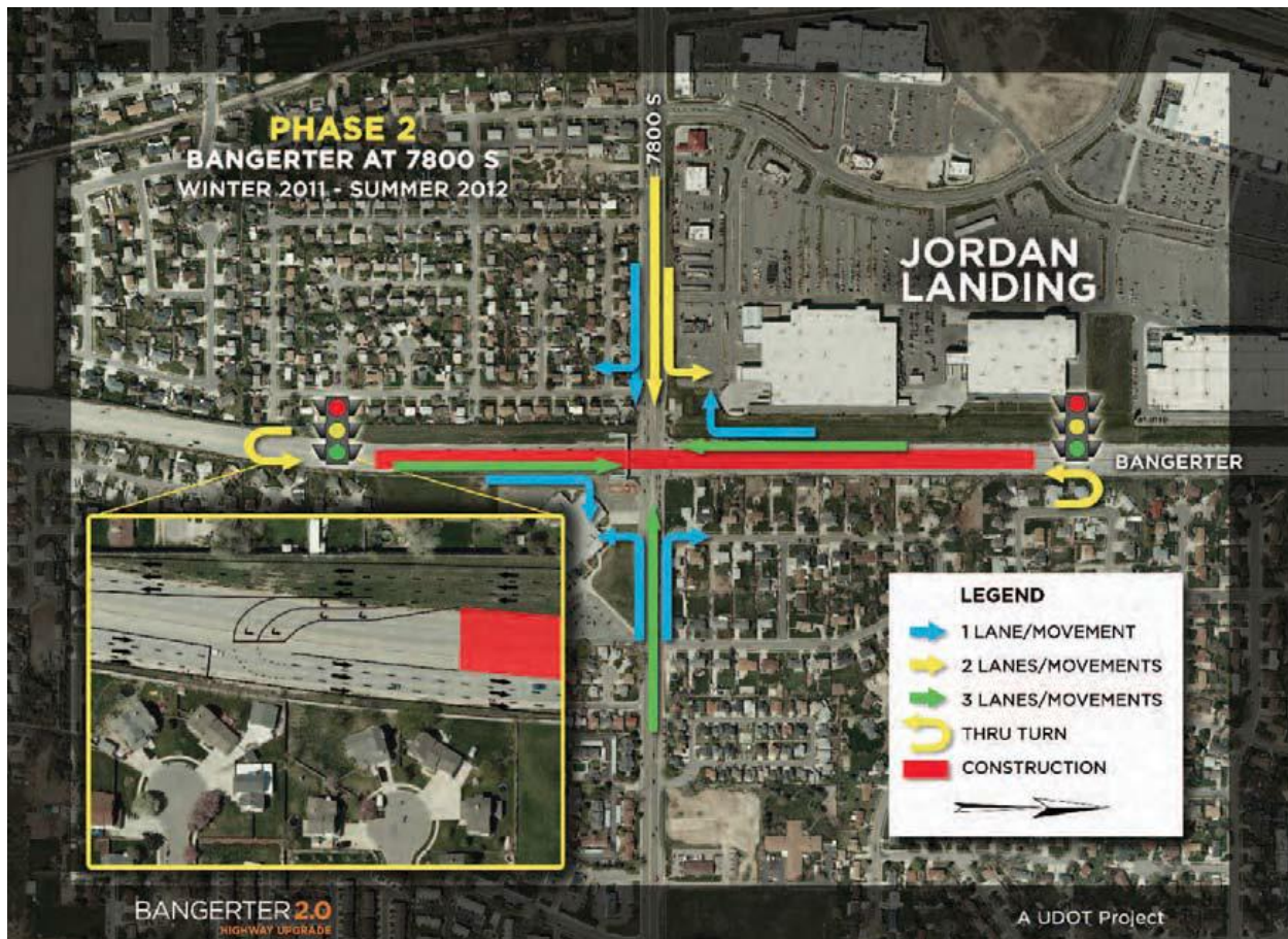
Figure C.2.1.3 Construction area and traffic movements for Phase 2 construction of SPUI at Bangerter Highway and 7800 South
