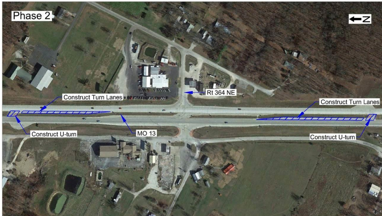
Figure C.4.1.3 Phase 2 construction of RCUT at MO 13 and Route 364 NE
