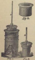
Fig. 1 represents the instrument entire. It consists of a sheet copper stand 8½ inches high, exclusive of the base, and 4½ inches in diameter. On one side is an aperture 3½ inches high for introducing a small spirit lamp, A, or better a small gasburner, instead of a lamp, when gas is available.
