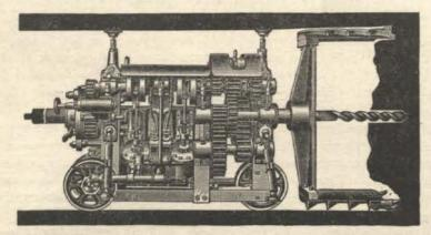
The accompanying cut shows the header at work in an entry. its cutting arms just entering the coal. This machine possesses great advantage in time and expense over ordinary methods of driving entries by hand. It makes more rapid progress, reduces the cost per foot of entry driven, leaves a firmer roof while driving it forward and reduces the cost of explosives.
