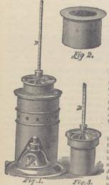
Fig. 1 represents the Instrument entire. It consists of a sheet copper stand \$3\forall inches high, exclusive of the base, and \$4\forall inches in diameter. On one side is an aperture \$3\forall inches high, for introducing a small spirit lamp, \$\mathbf{A}\$, or better, a small gas-burner, instead of a lamp, when gas is available.
