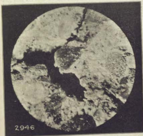
View showing lean and porous mortar. Under the microscope, the structure of the mortars and concretes of the pavement mixture examined, was strongly brought out. The view above shows a lack of cement sufficient to fill the voids in the sand, resulting in a very porous mortar. The above view is magnified about 30 diameters.
