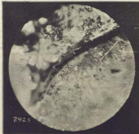
Photo micrograph, showing poor contact in mortar, mixed with porous pebbles. In this view a very porous aggregate pebble has absorbed the film of water which originally surrounded it, leaving a line of connected air voids around its circumference. Such a pebble, under traffic, will be quickly picked out or torn from the surface, and the mortar adjacent thereto will rapidly break down.
