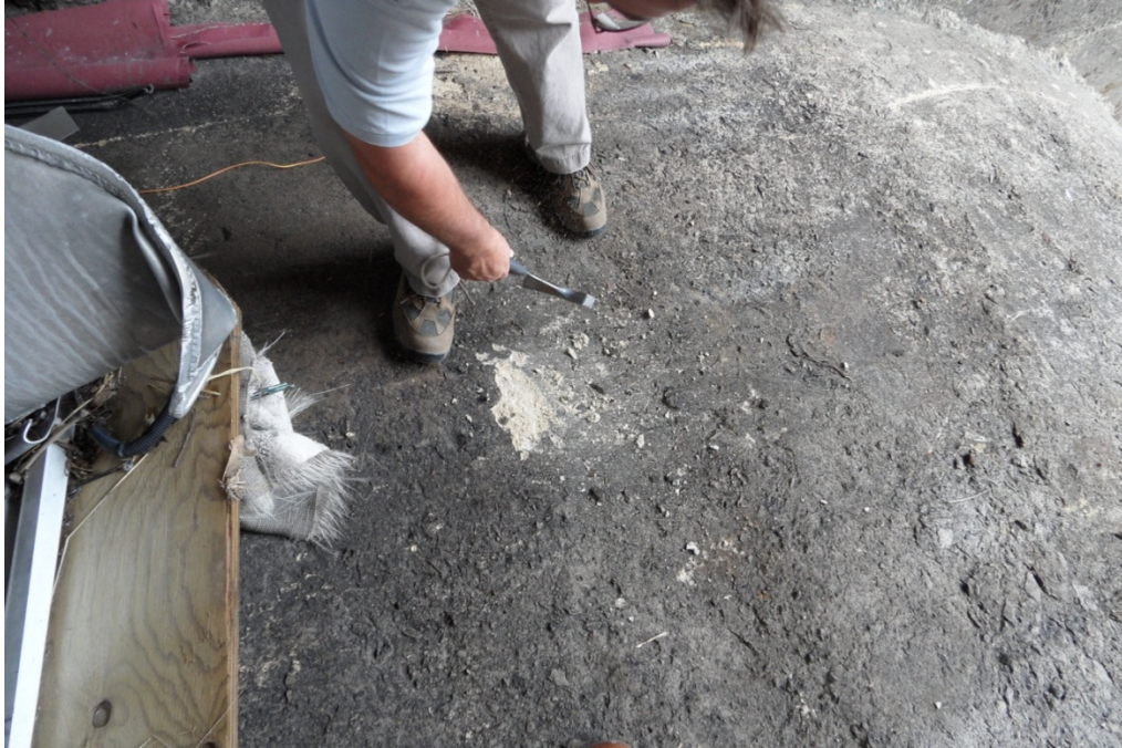
3.6 – Soft surfaces of spillway concrete can be chipped away with light hammer
