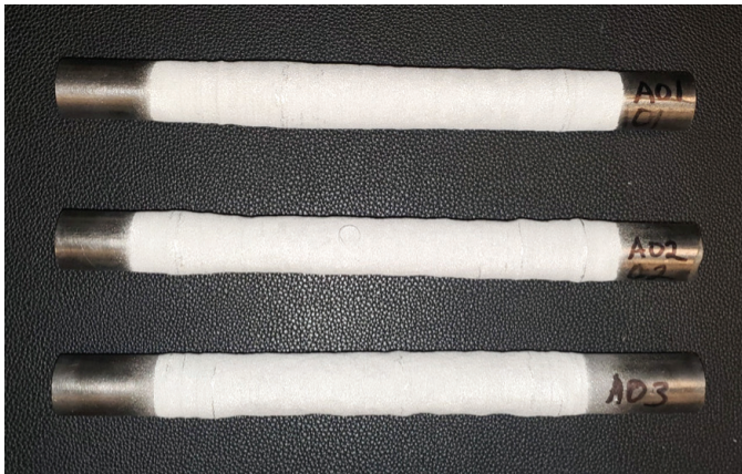
Steel coupons with the mass lost due to corrosion repaired using cold spray coating
