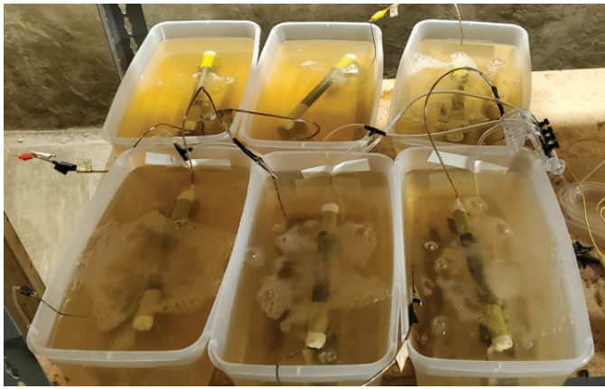
Accelerated corrosion testing on ASTM A36 steel coupons
