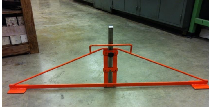
Figure 1. Deflectometer for measuring rutting
