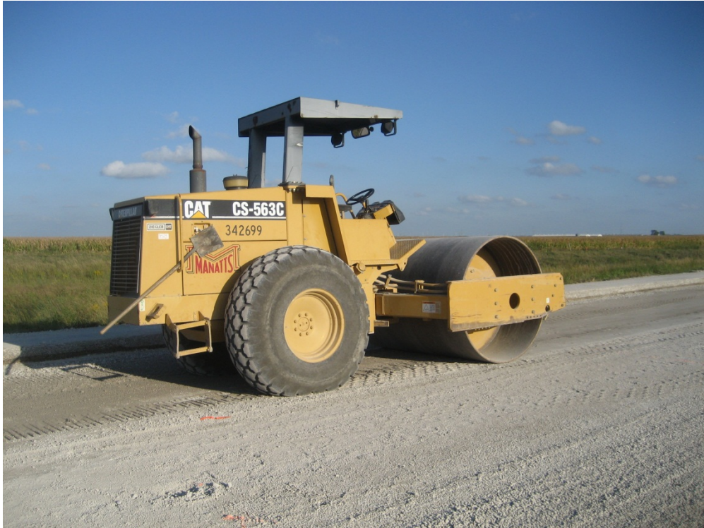
Figure 2. Self-propelled smooth drum roller used by contractor (non-vibratory)
