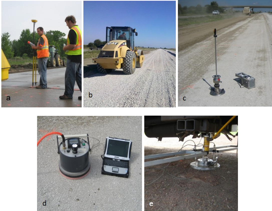
Figure 5. Trimble SPS-881 hand-held receiver (a), CAT CS683 smooth drum roller with CMV and MDP (b), Zorn LWD (c), gas permeability test (d), and static PLT (e)
