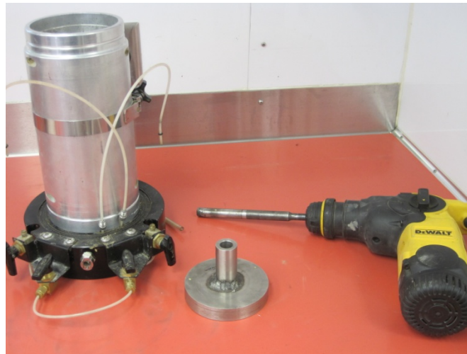
Figure 11. Split mold, steel platen (4 in. diameter), and vibratory hammer for compaction of granular materials
