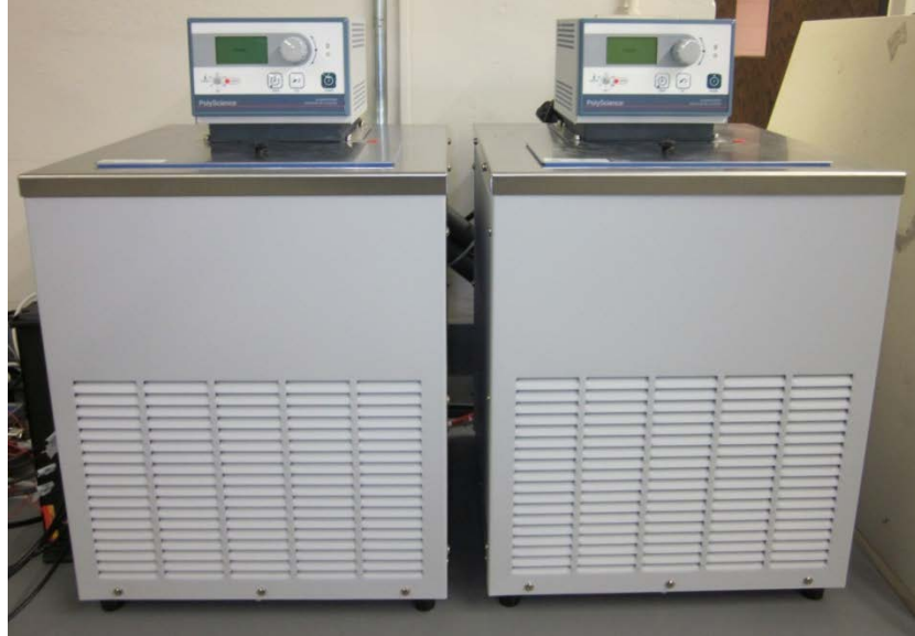
Figure 22. Temperature control water baths used to freeze and thaw samples
