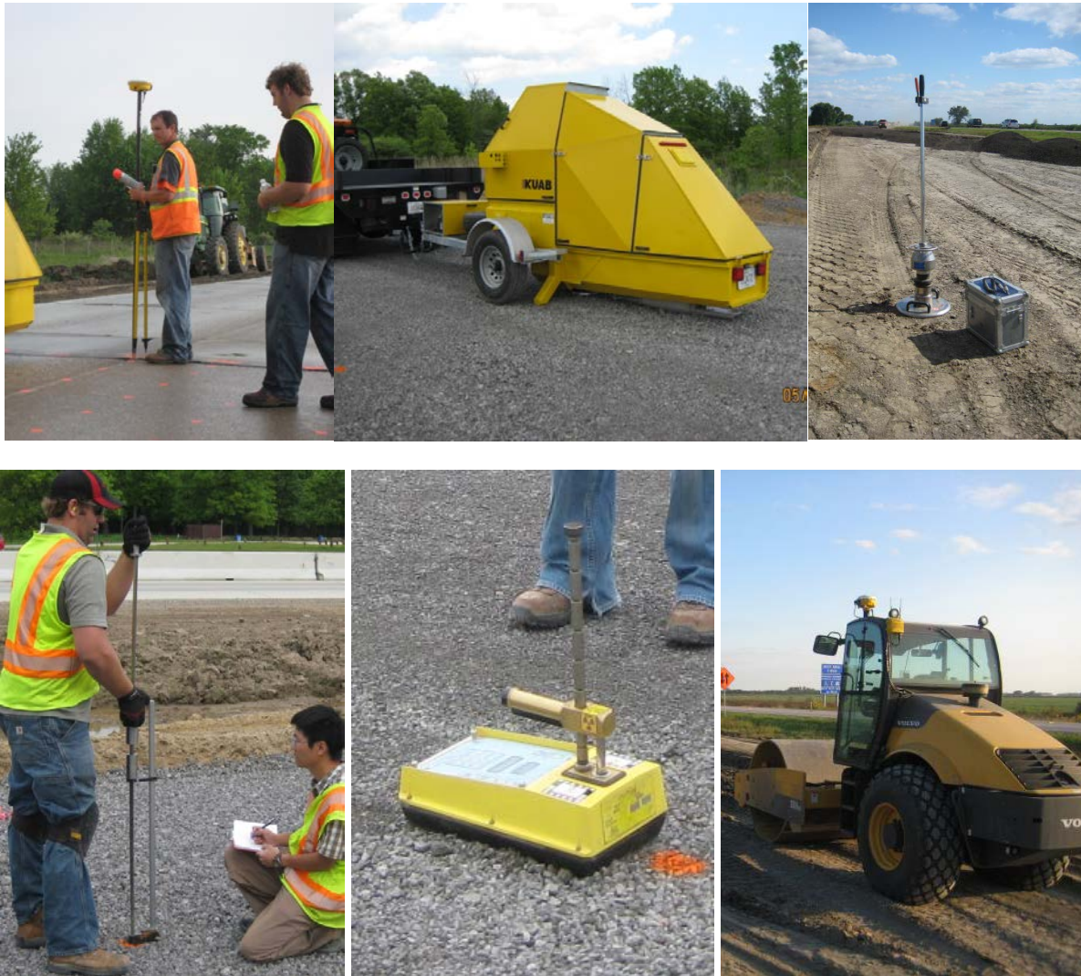
Figure 25. In situ test equipment: Trimble SPS-881 hand-held receiver, Kuab FWD, and Zorn LWD (top row left to right); DCP, NG, and Volvo smooth drum vibratory roller equipped with CMV measurement system (bottom row left to right)
