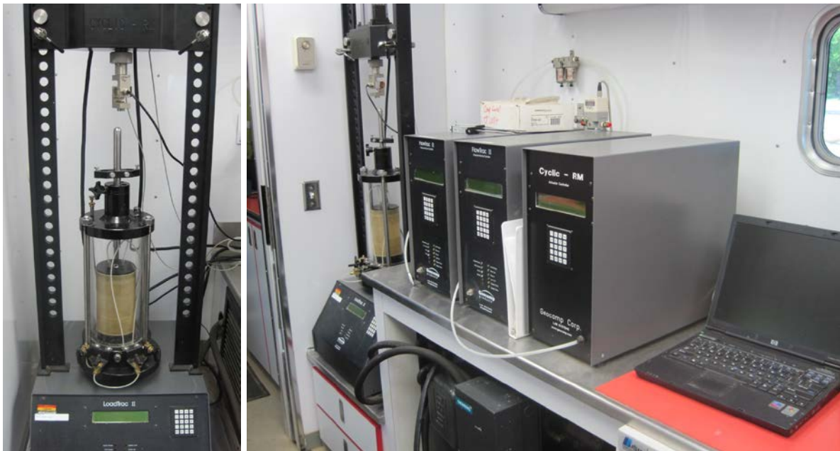
Figure 15. Triaxial chamber, load frame, and computer equipment for M_r testing
