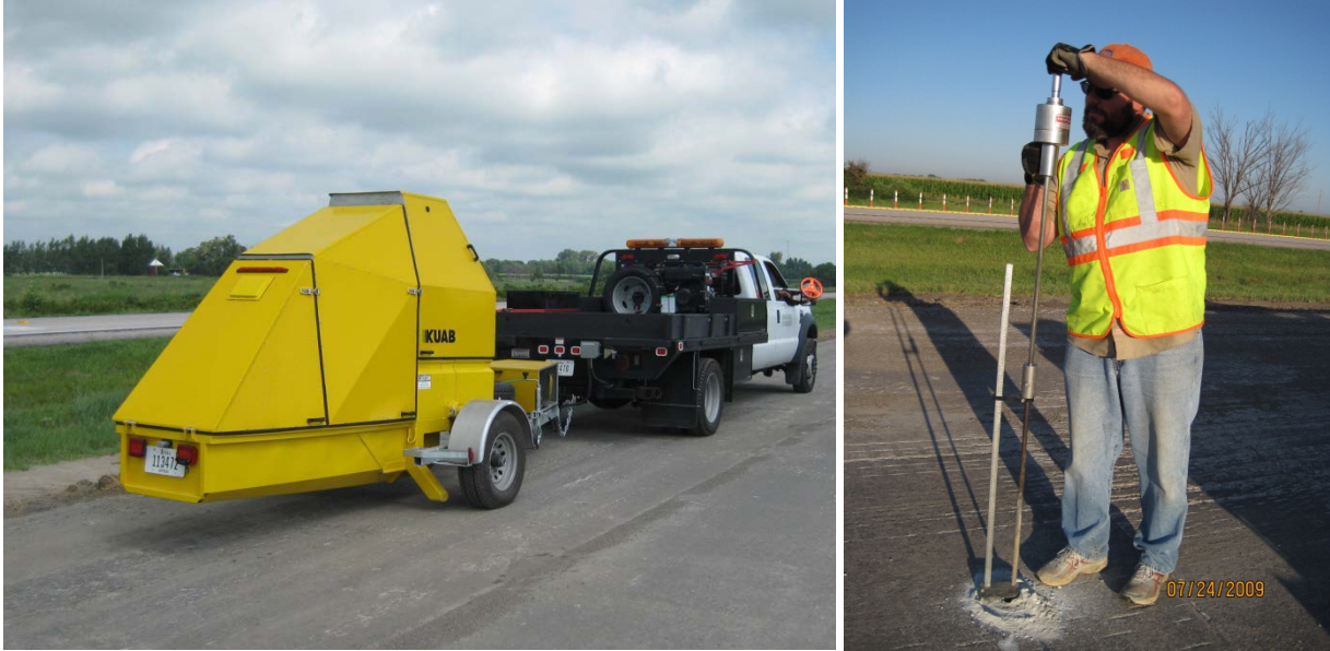
Figure 51. FWD and DCP testing on existing CRCP
