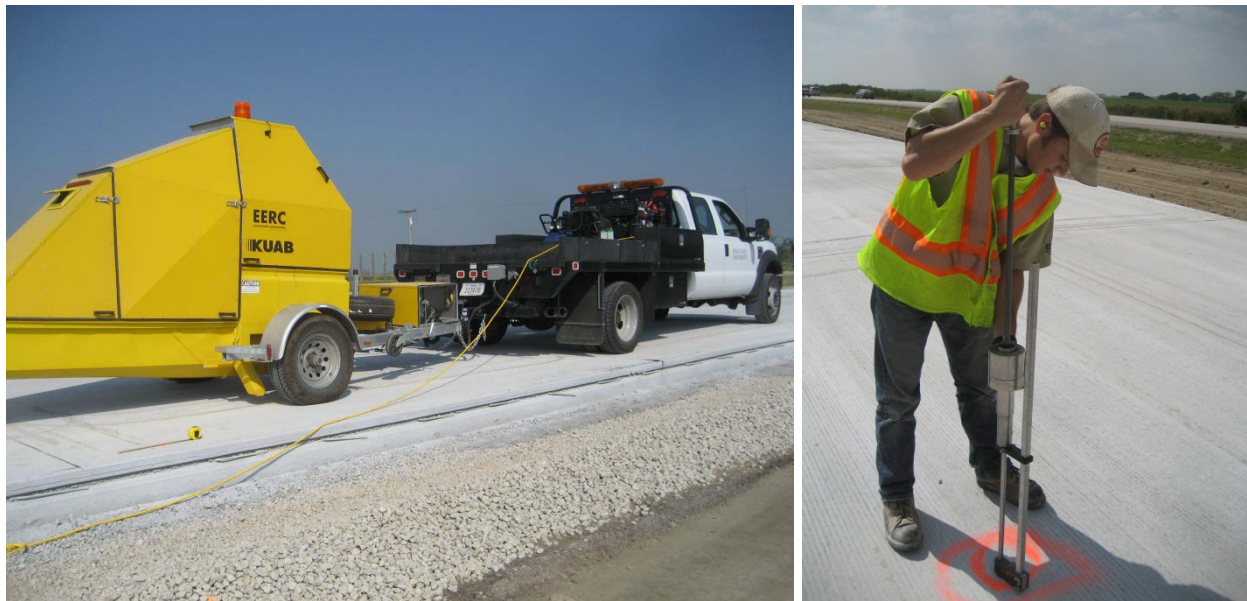
Figure 52. FWD and DCP testing on new JPCP
