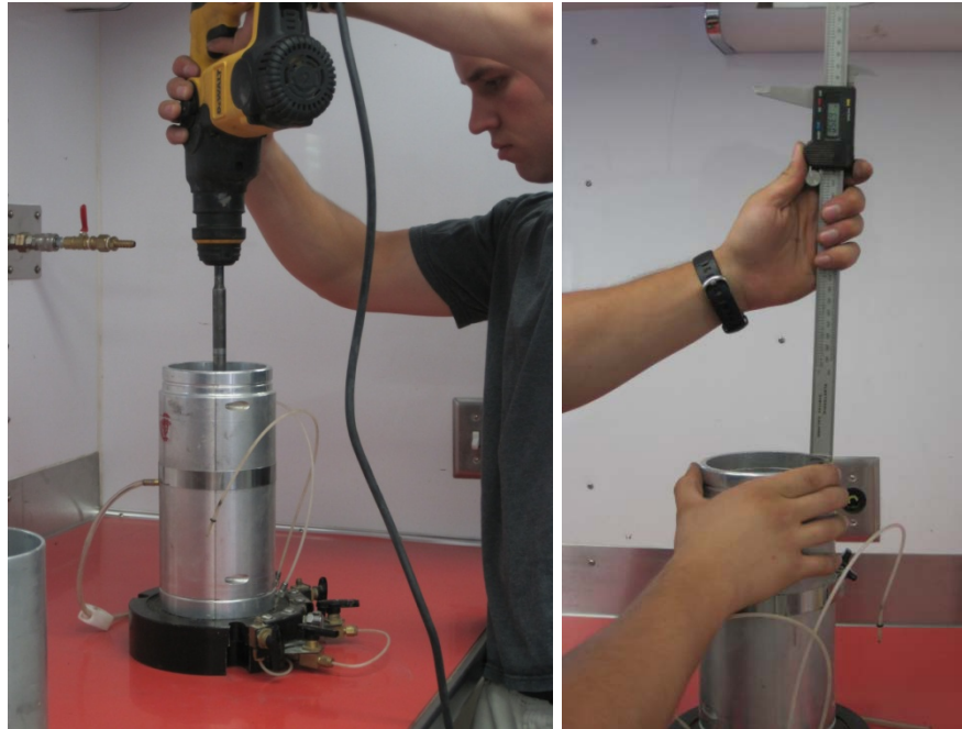
Figure 12. Compaction of granular materials in split mold (left) and verification of thickness of each lift using calipers (right)
