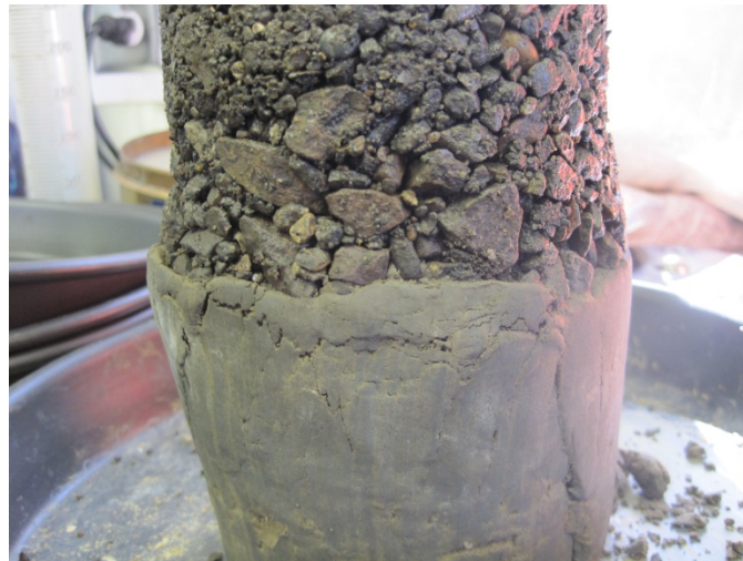
Figure 43. A photo of the recycled asphalt (18.82 kN/m 3 at w = 8.3\% ) over subgrade (17.29 kN/m 3 at w = 16.6\% ) layered composite sample after UU testing
