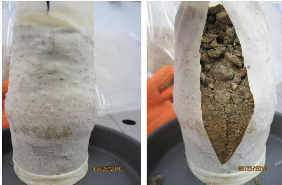
Figure 41. Photos of the RPCC (16.92 kN/m 3 at w = 5.7\% ) over select sand (21.41 kN/m 3 at w = 4.9\% ) layered composite sample after UU testing with the membrane intact (left) and open (right)
