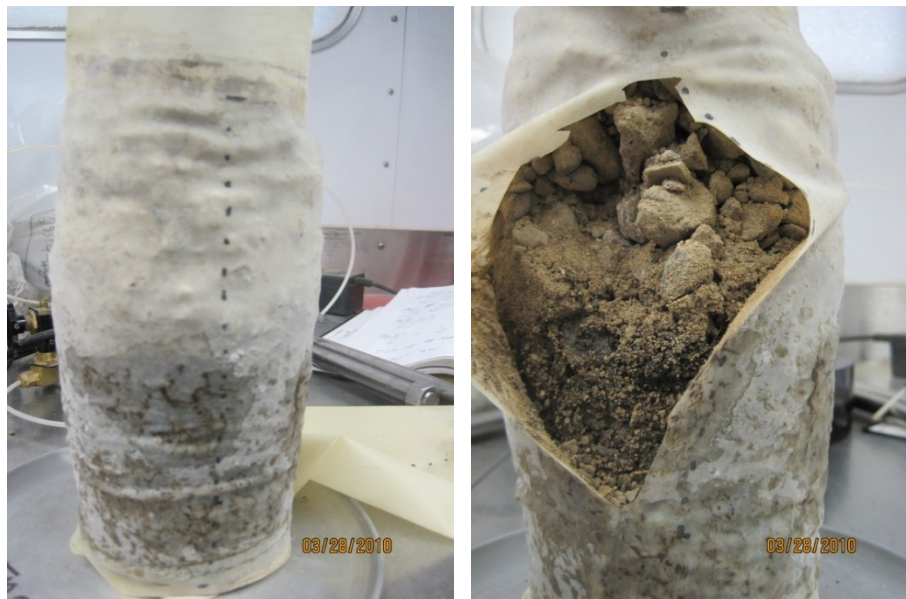
Figure 39. Photos of the RPCC (16.93 kN/m 3 at w = 4.9\% ) over recycled asphalt (19.94 kN/m 3 at w = 7.3\% ) layered composite sample after UU testing with the membrane intact (left) and open (right)
