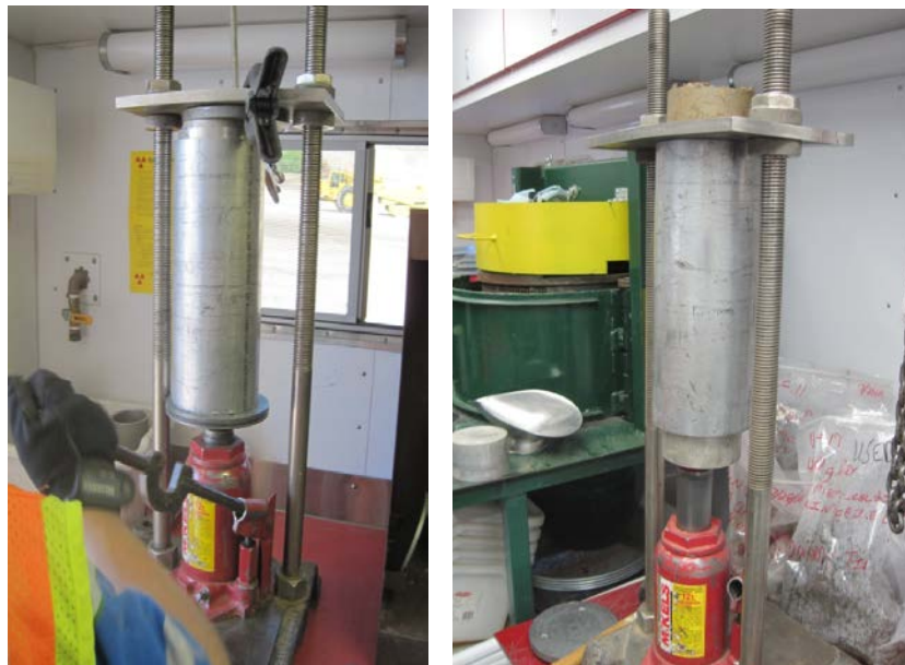
Figure 14. Photos showing static compaction procedure (left) and sample extrusion procedure (right) of a compacted cohesive soil sample
