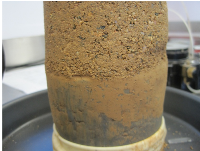
Figure 45. A photo of the select sand (21.13 kN/m 3 at w = 8.1\% ) over subgrade (17.39 kN/m 3 at w = 16.3\% ) layered composite sample after UU testing
