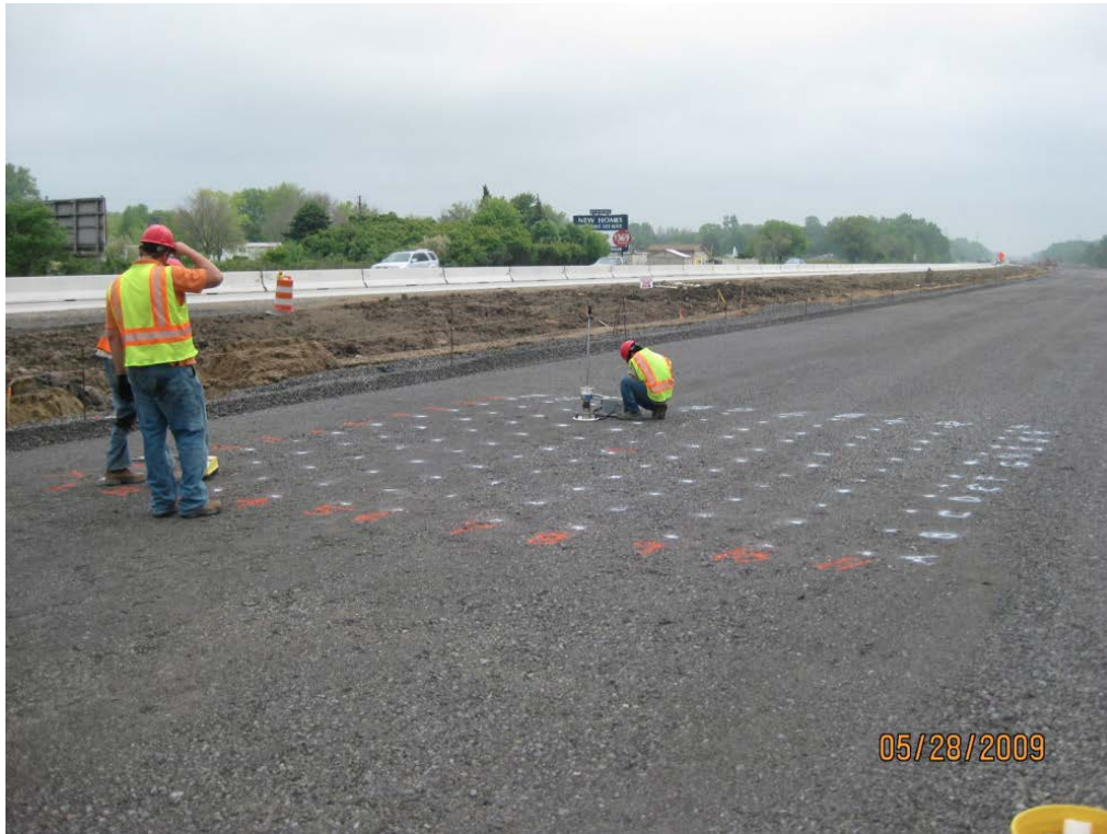
Figure 39. DCP test being carried out on an OGDC layer on TB1b (White et al. 2011)
