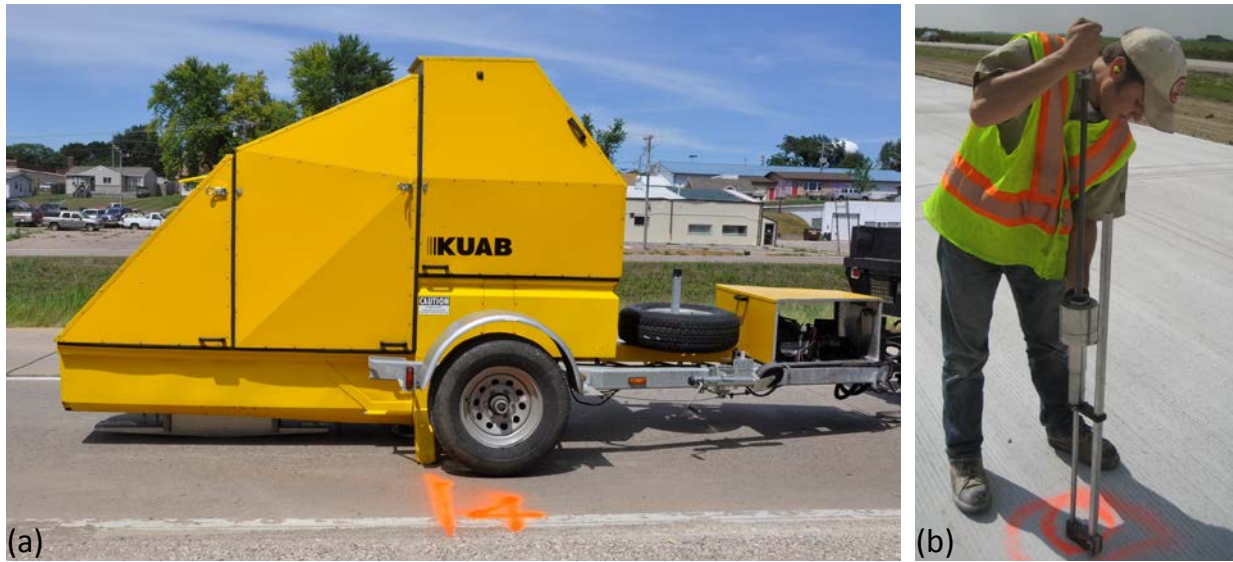
Figure 25. In situ testing procedures: Kuab FWD setup with 300 mm diameter loading plate (a) and DCP with 2m extension rods (b)
