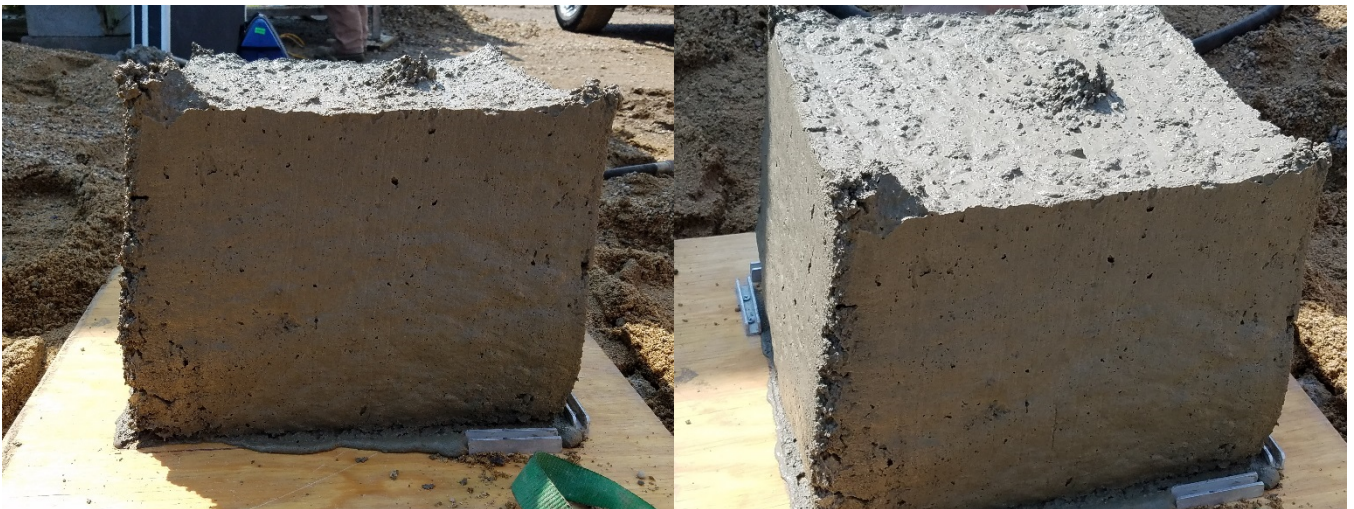
Figure 5: Box Test PEM Shoulder Mix
