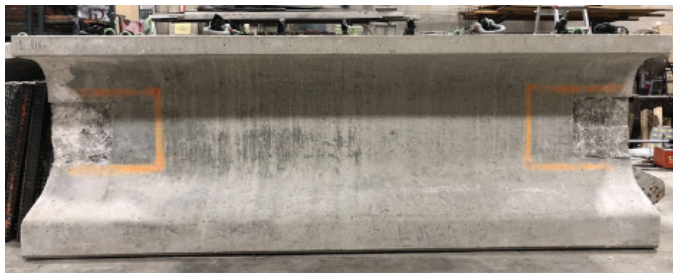
Beam specimen with artificial damage on both ends
