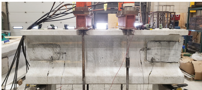
Patched beam specimen instrumented for the four-point bending test
