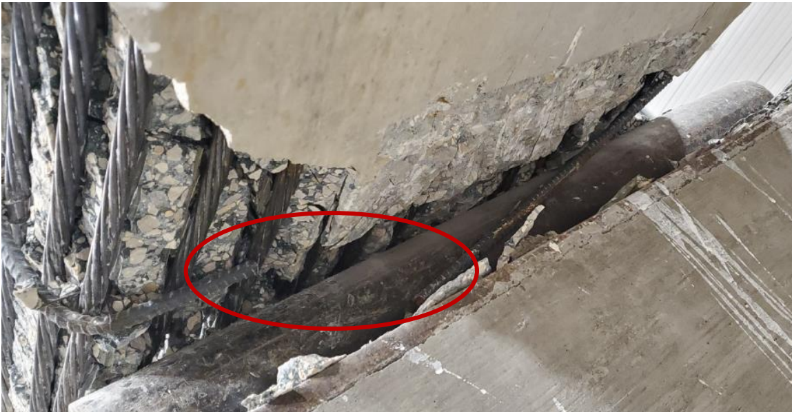
Figure 4.14. Fractured stirrup on bottom flange of Control-2
