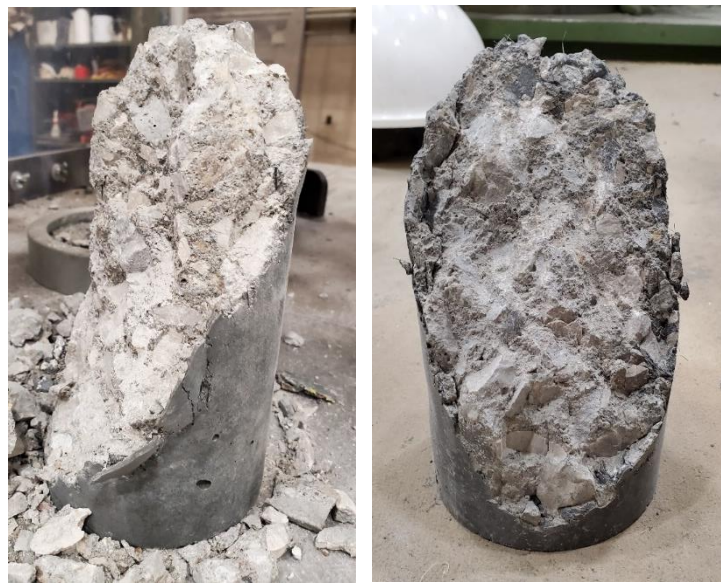
Figure 3.12. Examples of failed UHPC slant shear specimens
