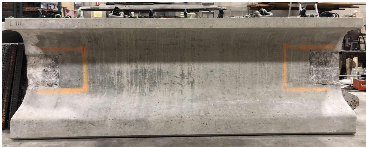
Figure 4.6. Artificially damaged beam specimen (1 ft damage)
