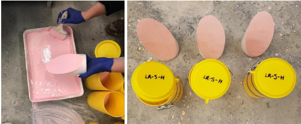
Figure 3.2. Formwork retarder application
