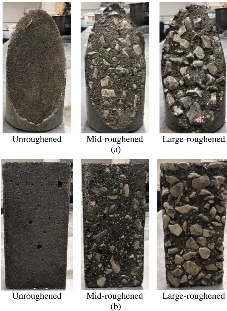
Figure 3.3. Various levels of surface roughness for the substrate specimens: (a) slant shear specimens and (b) splitting tensile specimens
