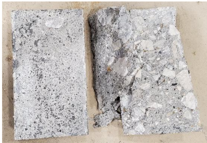
Figure 3.9. Example of UHPC-NP specimen after failure
