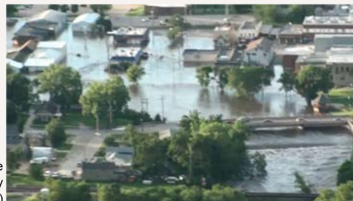
Manchester, Flood of 2010. When a dam's influence is clearly visible during a flood, like the dam below the bridge in Manchester, the dam likely contributes to upstream flooding. (Photo from AP video footage.)
