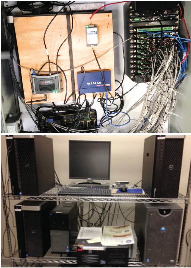
Typical Bridge Engineering Condition Assessment System (BECAS) computer hardware arrangement: field installation in a cabinet on-site (top) and data processing cluster in the office (bottom)
