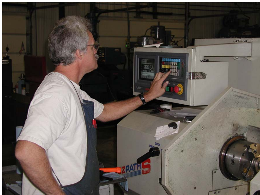
Photo above: Jim Matheny, machinist, programs a CNC lathe at Iowa Tool and Manufacturing, Inc. in Creston.
