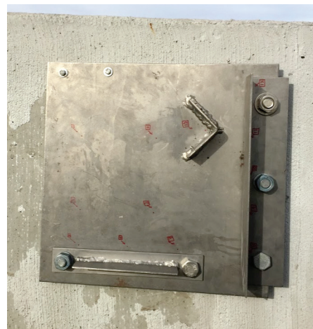
A1010 steel plate with stainless steel and galvanized steel bolts and welded connection
