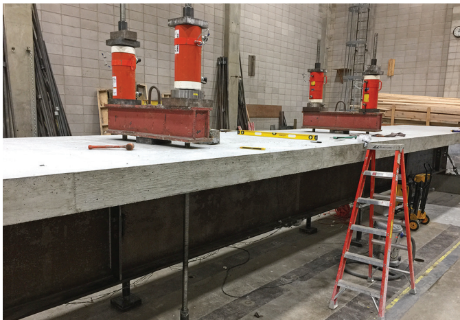
Loading setup for composite beam under 50% yield moment
