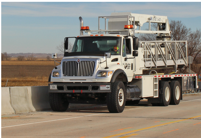
Live-load testing on the bridge
