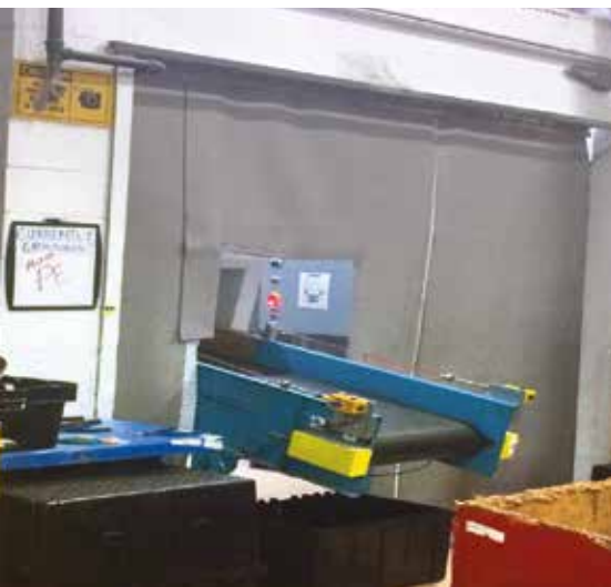
Gray sound-dampening curtains quieted the Orbis Corporation granulator.
