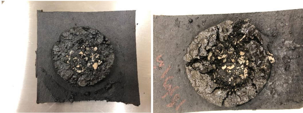
Figure 8. Modes of emulsified asphalt rupture: “solid spin” (left) and “normal” (right)
