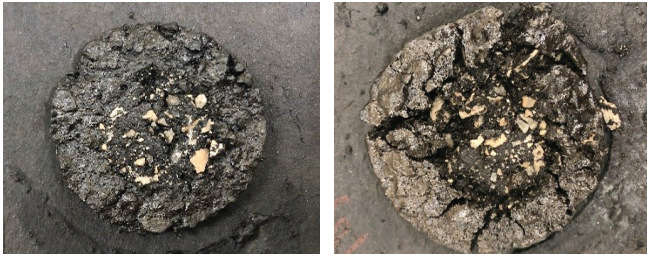
Examples of modes of emulsified asphalt rupture: “solid spin” (left) and “normal” (right)
