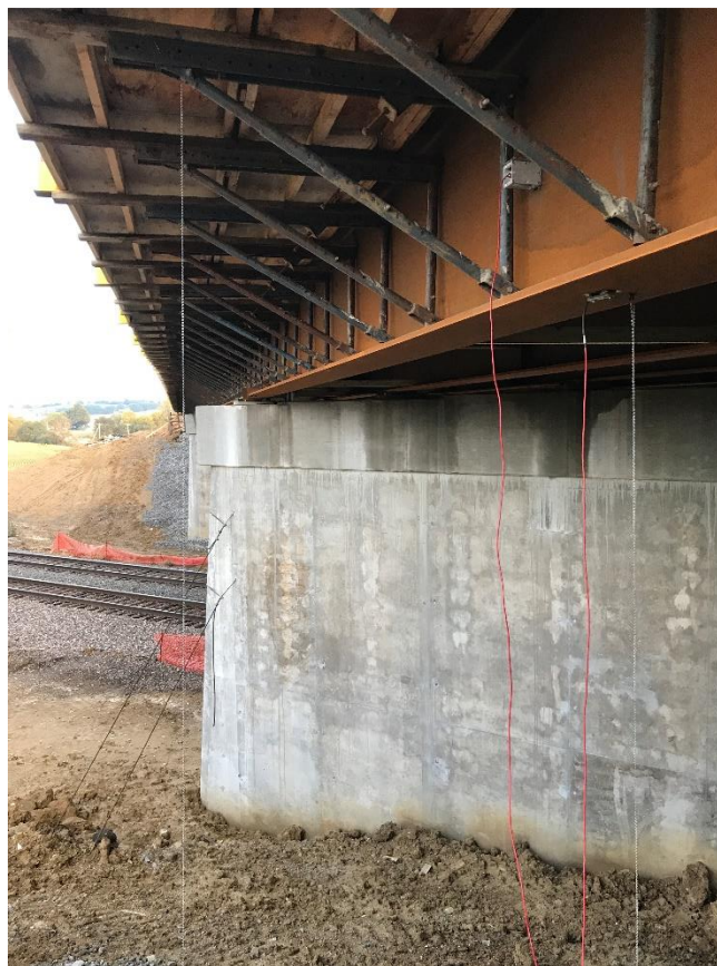
Figure 40. BNSF Railway Bridge exterior girder field instrumentation
