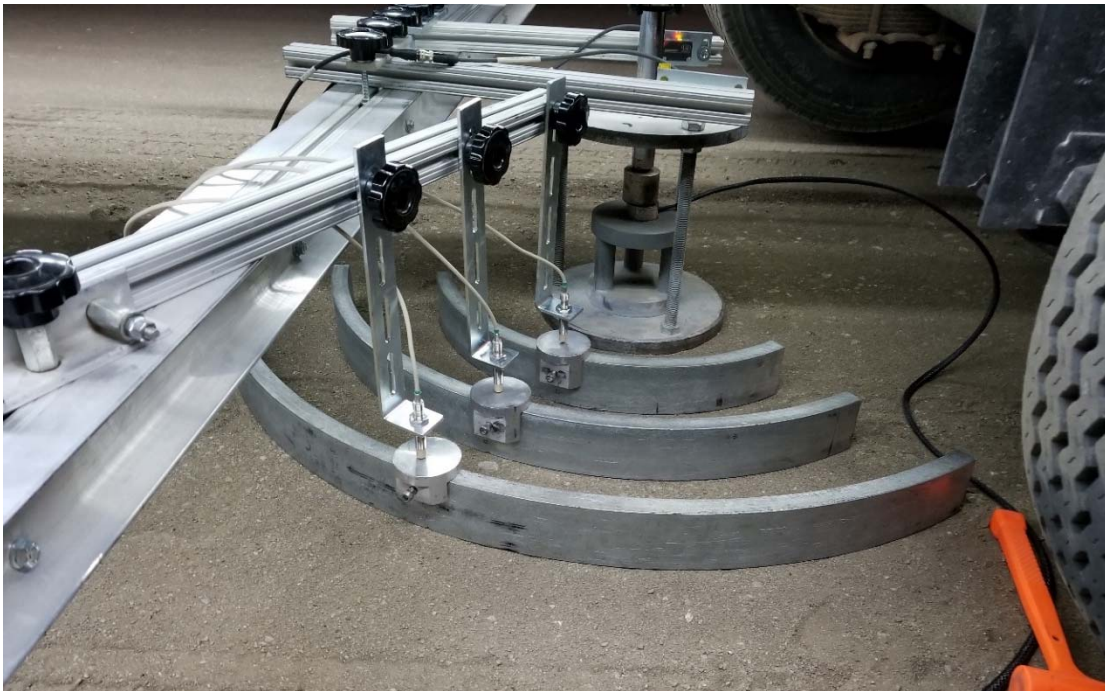
Figure 9. 12 in. diameter loading plate setup for cyclic APLT on Project 3 – I-35/US30E Ramp (picture taken on 10/28/2017).
