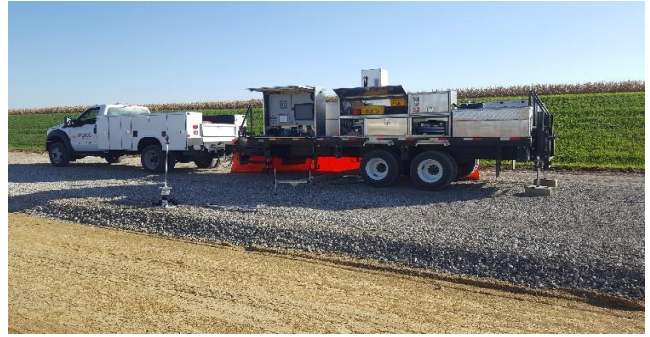
Measurement of granular subbase layer thickness
