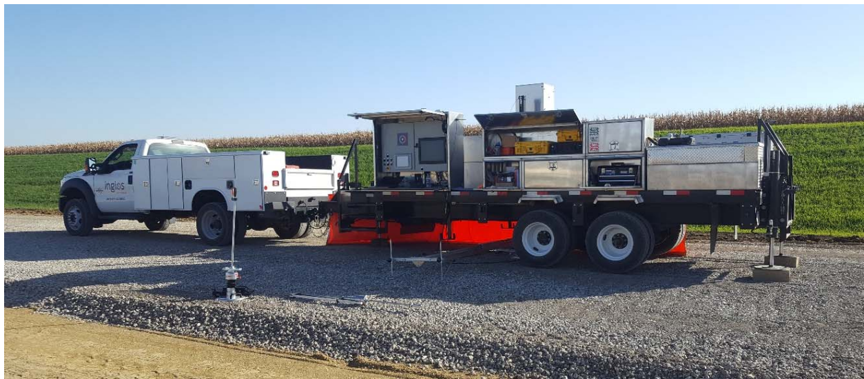
Figure 2. Automated plate load testing setup from Project 2 – US 20 (picture taken on 10/19/2017)
