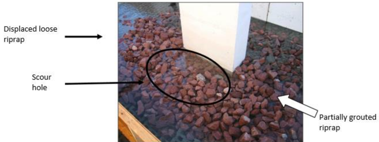
Figure 8. Laboratory test results on loose and partially grouted riprap
