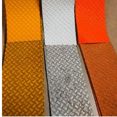
Figure 40. Comparison of yellow, white, and fluorescent orange tapes when new (upper samples) and after approximately 3½ months in the field (lower samples)
