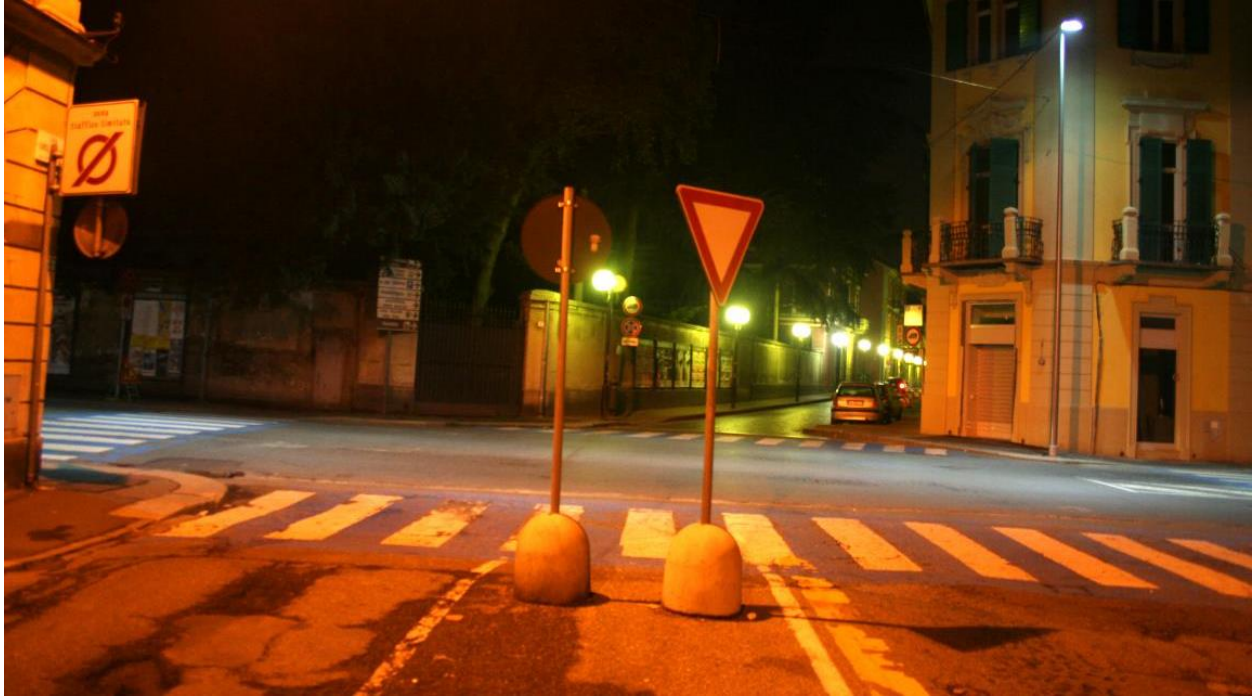
Figure 31. Comparison of color effects of three roadway lighting technologies. Foreground: high-pressure sodium (pinkish orange). Crosswalk and intersection: LED (bluish white). Side street in background: Mercury vapor (greenish)
