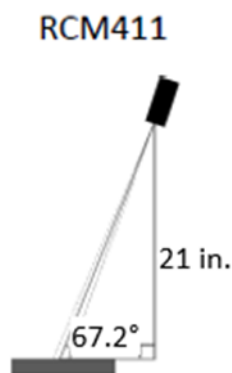
Figure 7. Recommended mounting height and angle for the Teconer RCM411
