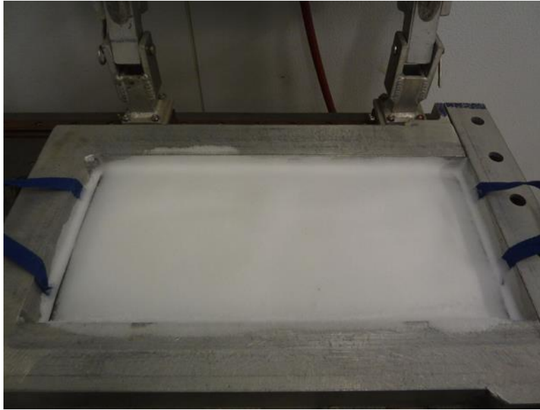
Figure 12. Pavement sample with compacted snow in the compaction machine
