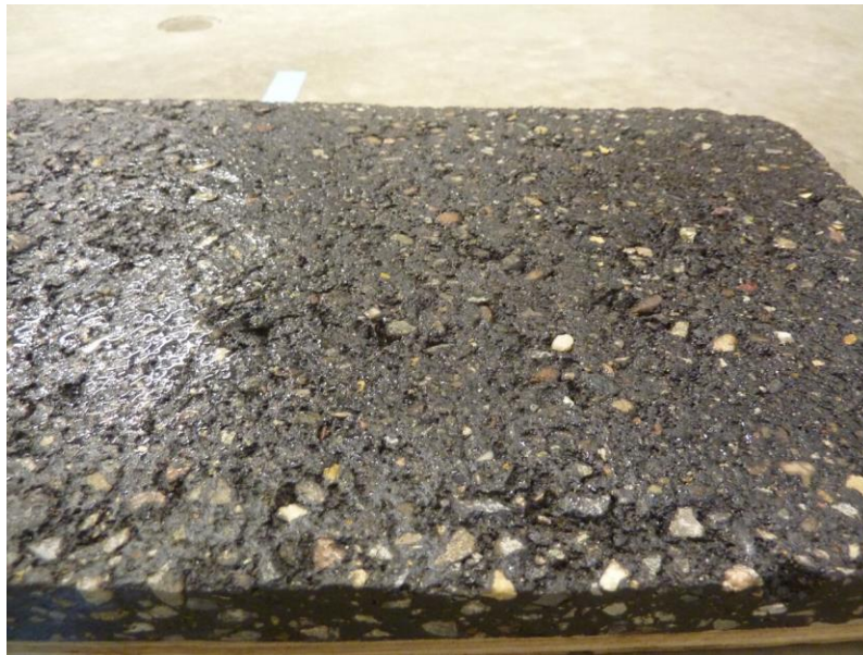
Figure 11. Asphalt sample with salt brine applied
