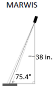
Figure 8. Recommended mounting height and angle for the MARWIS
