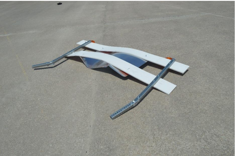
Figure 64. System Damage –Test No. WZNP-1, System B
