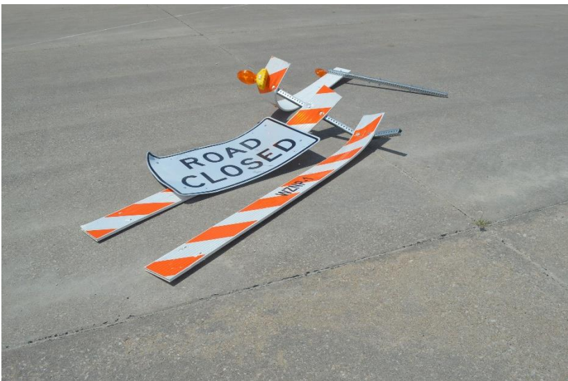
Figure 63. System Damage –Test No. WZNP-1, System A
