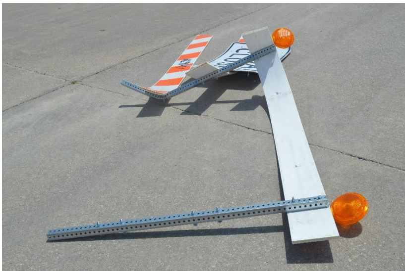
Figure 63. System Damage –Test No. WZNP-1, System A
