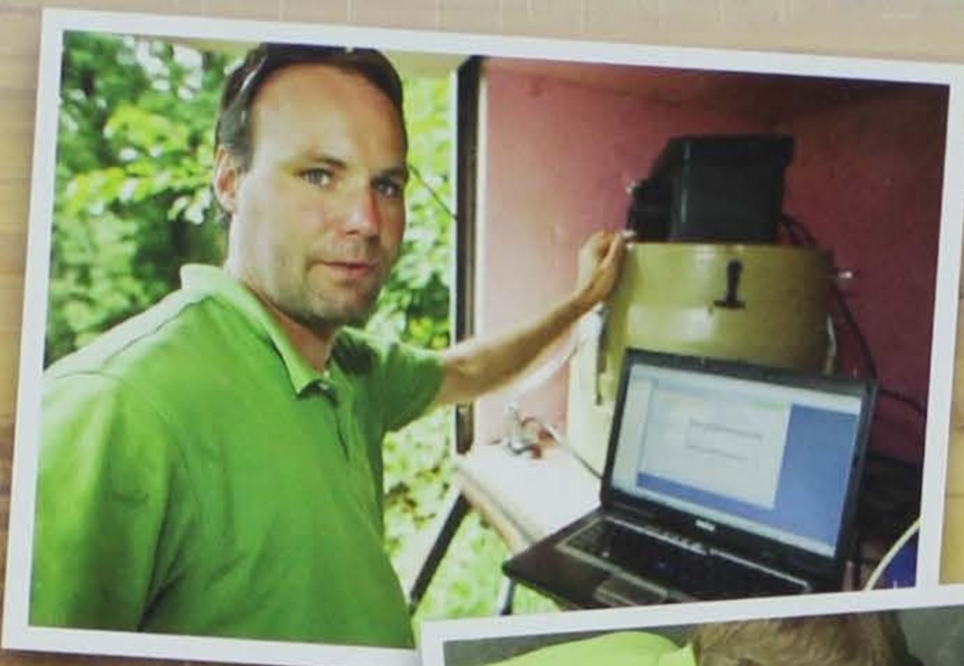
Water quality technician Tony Seeman of the Iowa Soybean Association makes weekly visits to field stations to collect water samples and data. The information helps determine how quickly water and nitrogen infiltrates fields to enter drainage tiles below ground.
