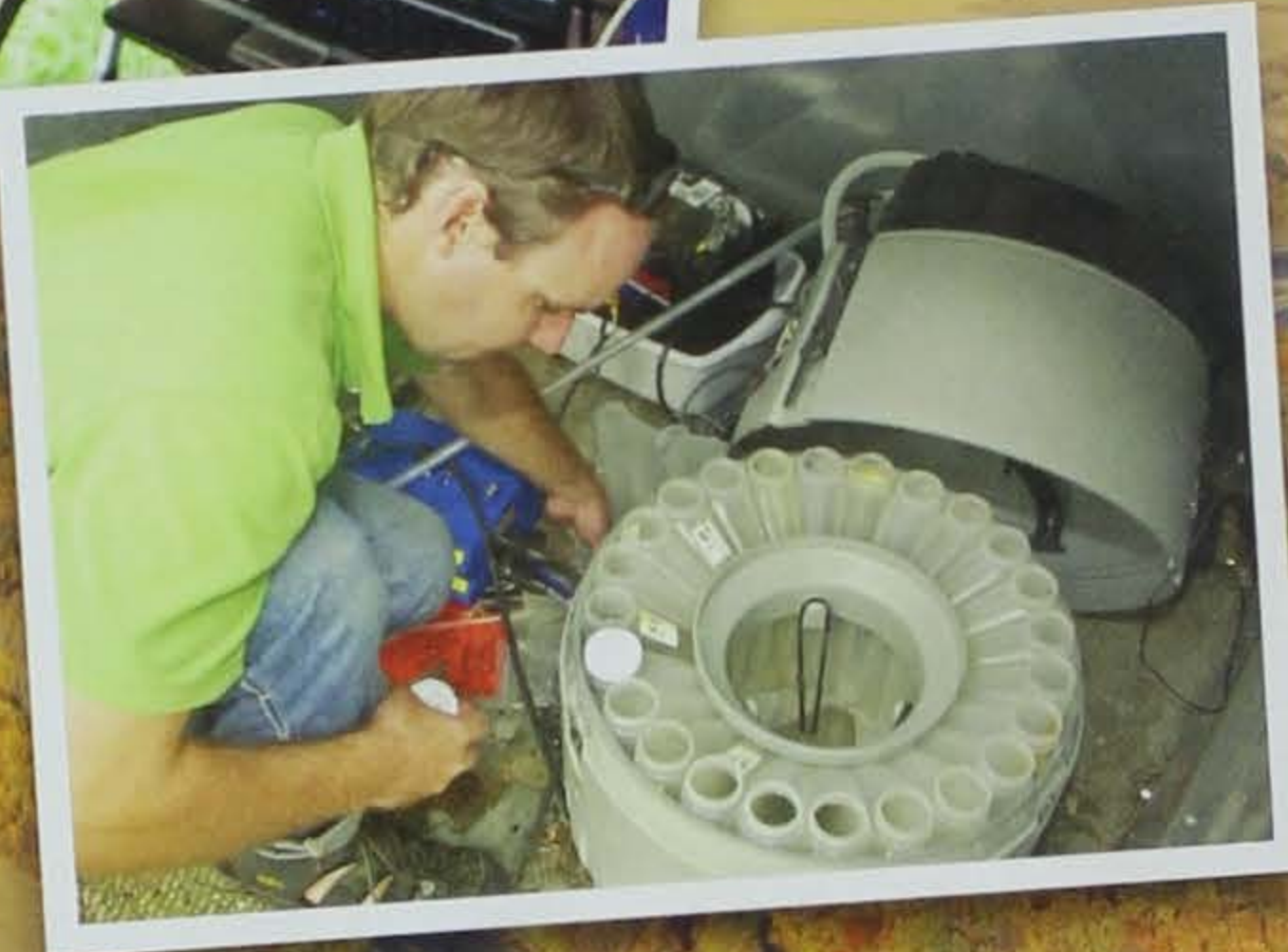
Water quality technician Tony Seeman of the Iowa Soybean Association makes weekly visits to field stations to collect water samples and data. The information helps determine how quickly water and nitrogen infiltrates fields to enter drainage tiles below ground.
