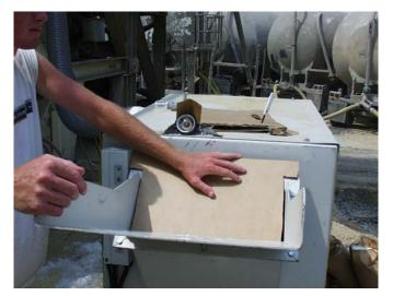
Figure 14. Adjustment to Blower for Better Fiber Dispersion
