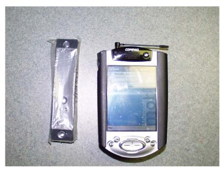
Figure A.6. IRD Concrete Maturity Monitor (International Road Dynamics)
