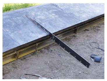
Figure 11. Longitudinal Joint Forming Knife
